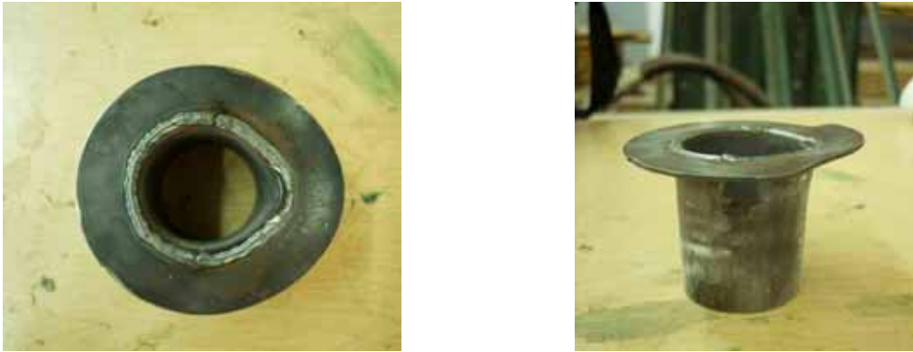
Figure 2.10 Deformation to Bottom Sleeve
