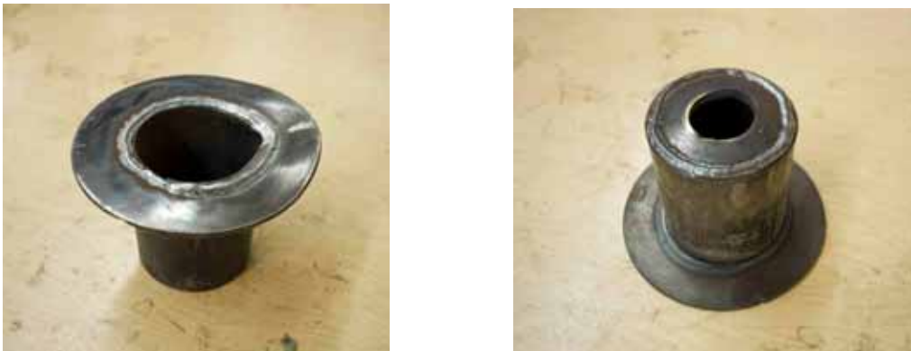
Figure 2.9 Deformation to Outside and Inside Washer of Top Steel Sleeve
