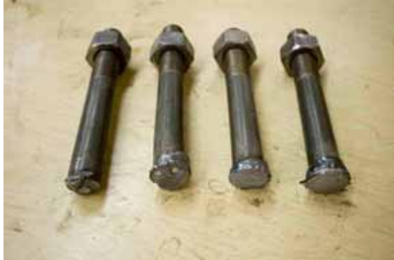
Figure 2.15 Fracture of Shear Stud
