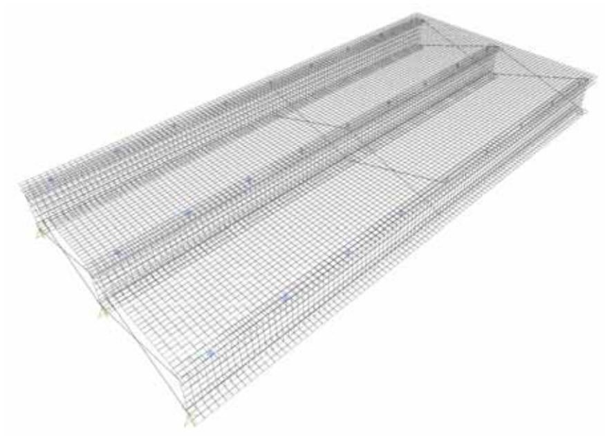
Figure 4.3 FE Bridge Model
