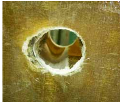
Figure 2.12 Bottom Facesheet at Failure
