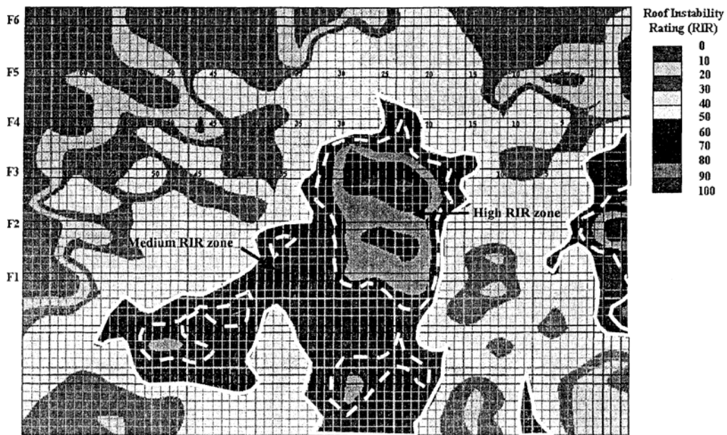
Figure 2.13 Roof Instability Rating (after Stankus et al., 2001)
