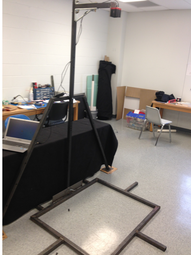
Figure 25: Final construction of test apparatus, with SwissRanger attached.
