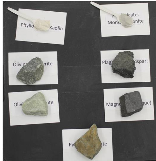
Figure 26: Sampling of minerals on containment tray for integration time determination. Row 1: kaolin, montmorillonite. Row 2: Coarse grained forsterite, augite. Row 3: Fine grained forsterite, magnetite. Row 4: augite
