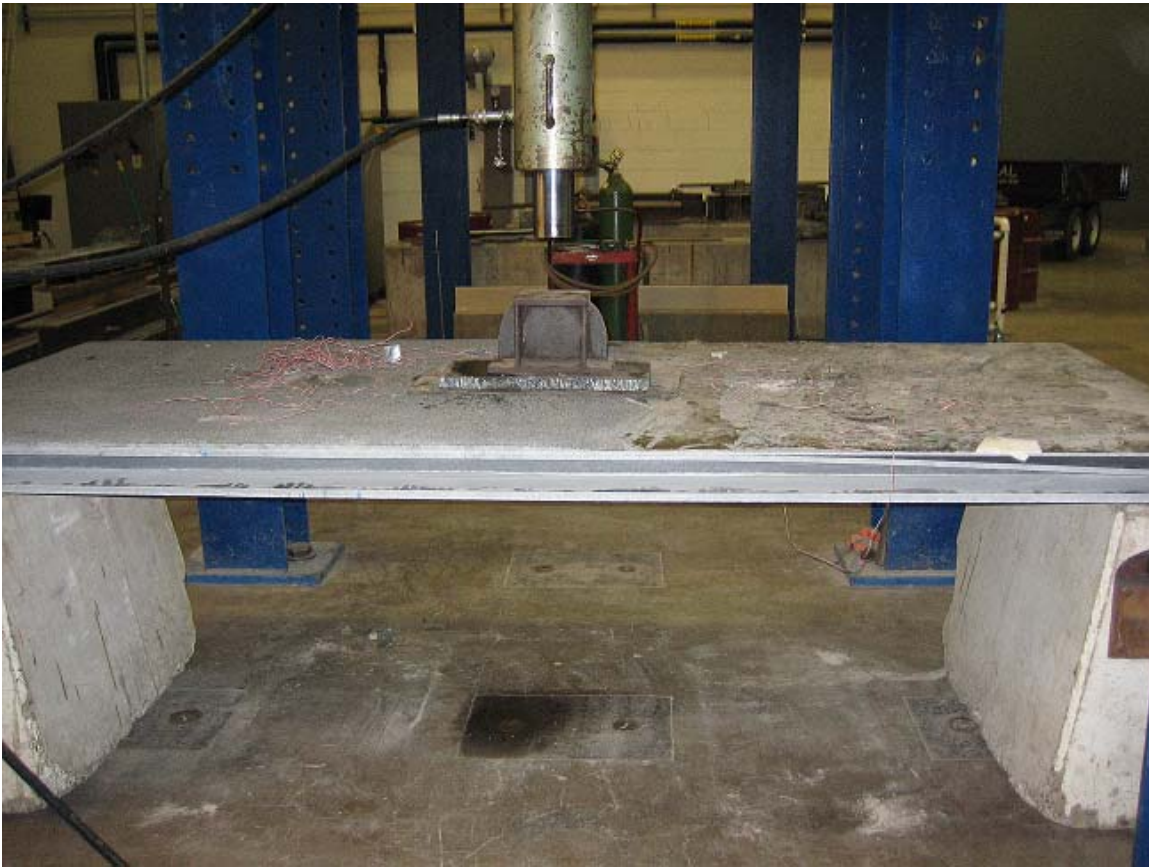
Fig. 6.2 Test set-up for 2 module FRP deck component
