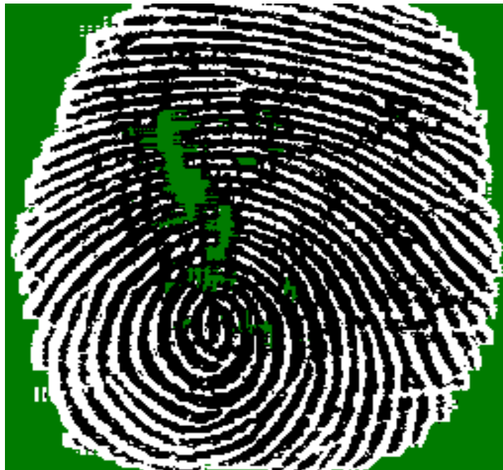
Figure II-12. Image showing a fingerprint that has been outlined with the masked pixels shown in green. The image has also been converted to binary.
