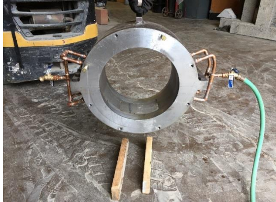
Figure 5-22: the hollow shell with cooling chamber.
