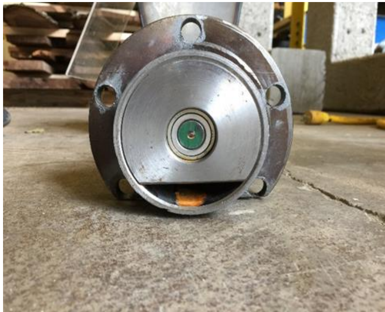
Figure 5-4: Opening on one end of the Screw Auger.
