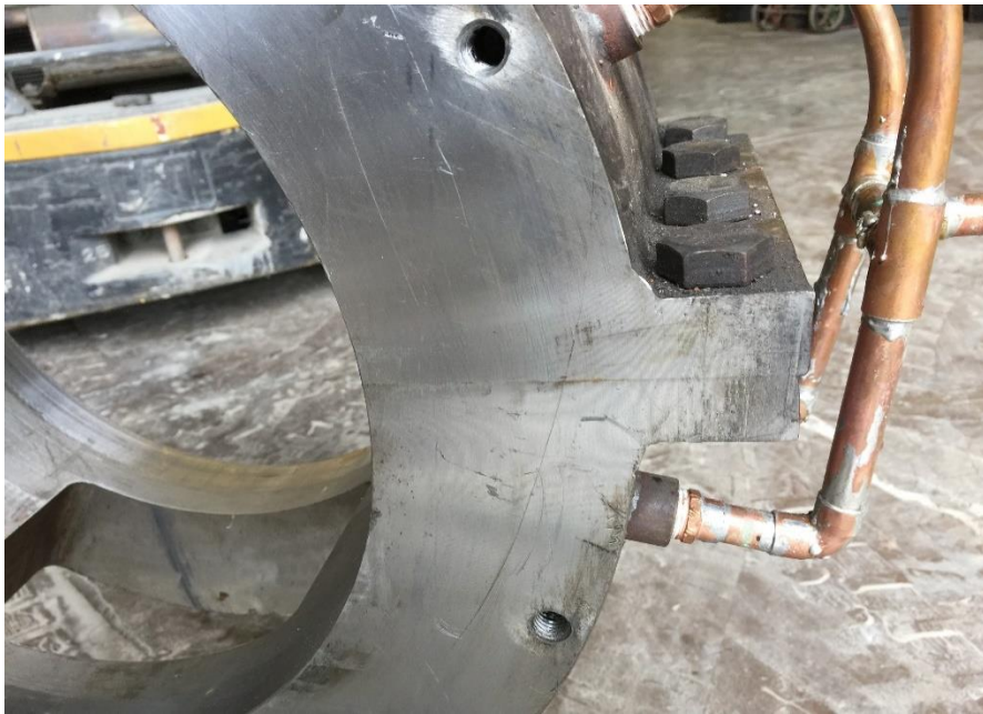
Figure 5-12: Semi Circular components bolted and welded together to form cylindrical chamber.
