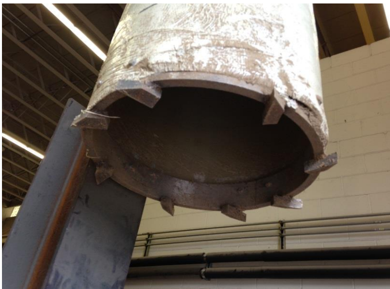
Figure 3-8: Cutting teeth with the cutting edge.
