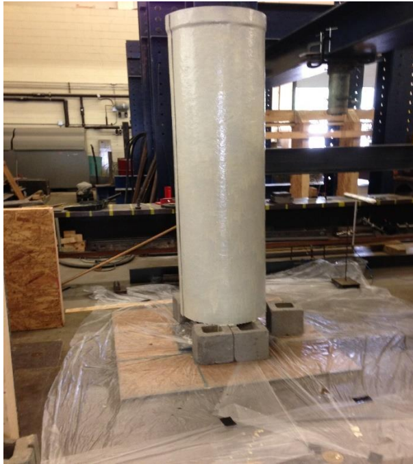
Figure 4-1: Simpsons Strong-TieFx-70 jacket.
