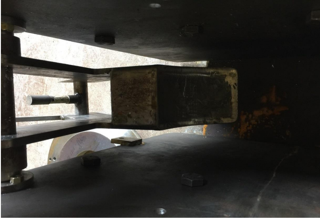
Figure 5-14: Dumping arm attached to parallel plates.
