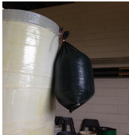
Figure 3-15: Sand bags Used to apply Vertical loads.
