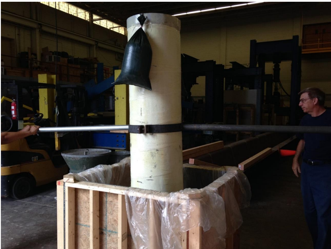
Figure 4-13: Hollow cylindrical tube to produce torque.
