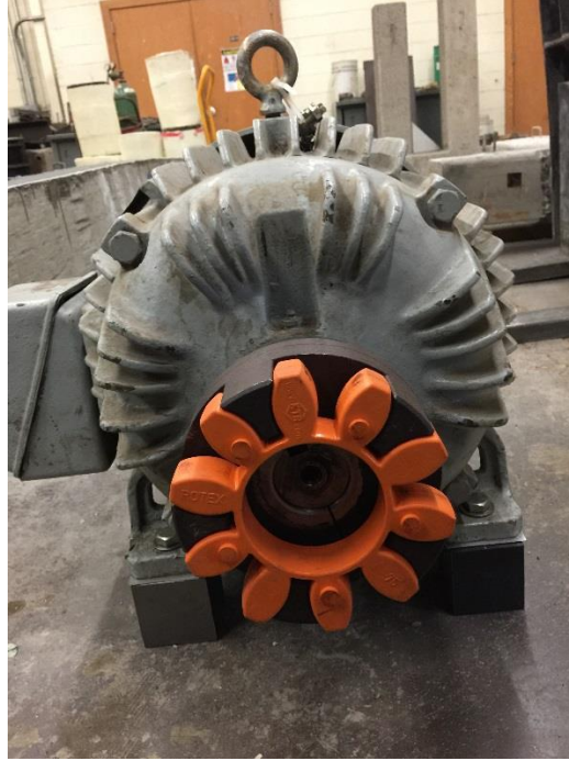
Figure 5-21: Coupler on the motor shaft.
