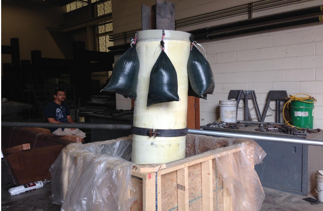
Figure 4-15: FRP shell bored down into the soil.
