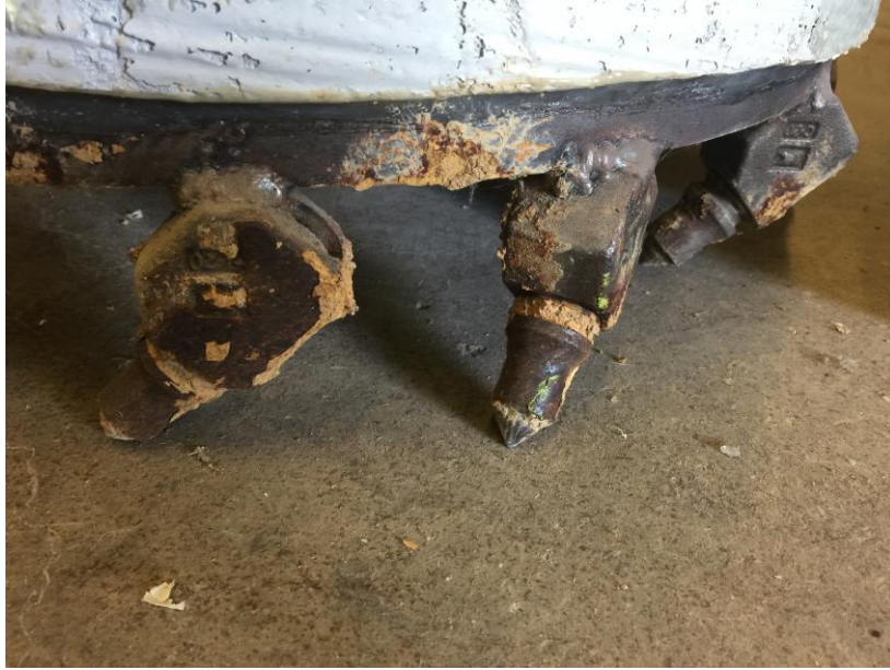
Figure 3-11: Bullet teeth with the blocks attached to the circular ring.
