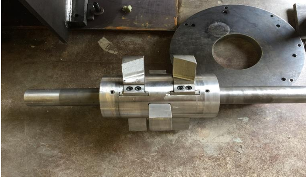
Figure 5-11: Shaft with grinding teeth.
