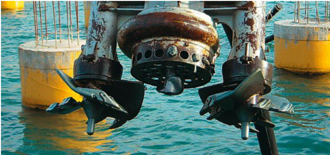
Figure 2-9: The suction pump with the agitators (ABC Diving® , 2016).
