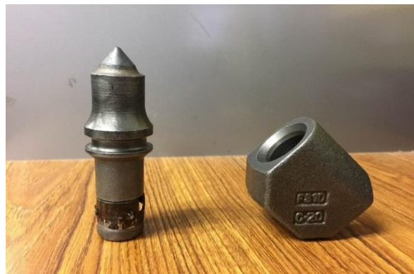
Figure 3-10: Conical bullet teeth and block holder.
