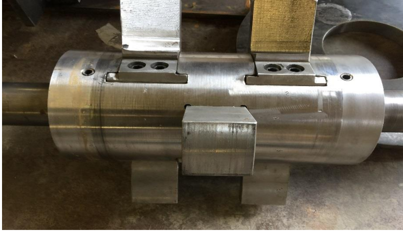
Figure 5-16: Portion of shaft that remains inside the heating chamber.
