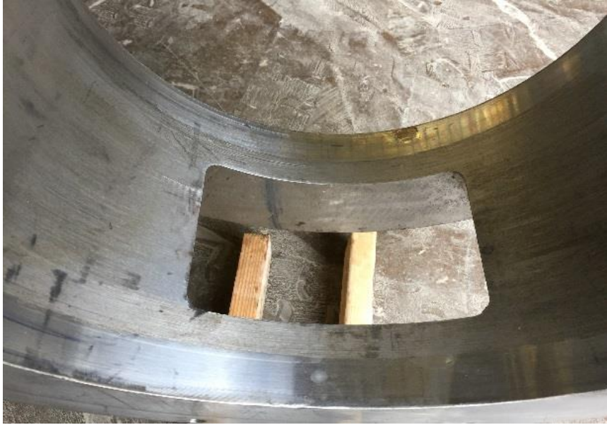
Figure 5-9: Opening for dump door.
