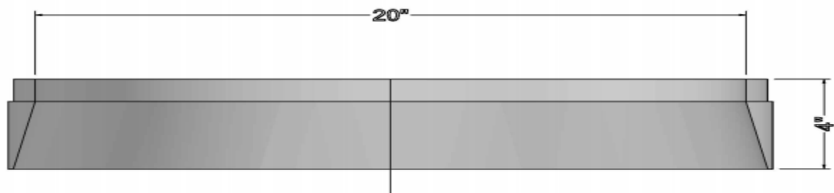
Figure 3-2: Arched member front view.
