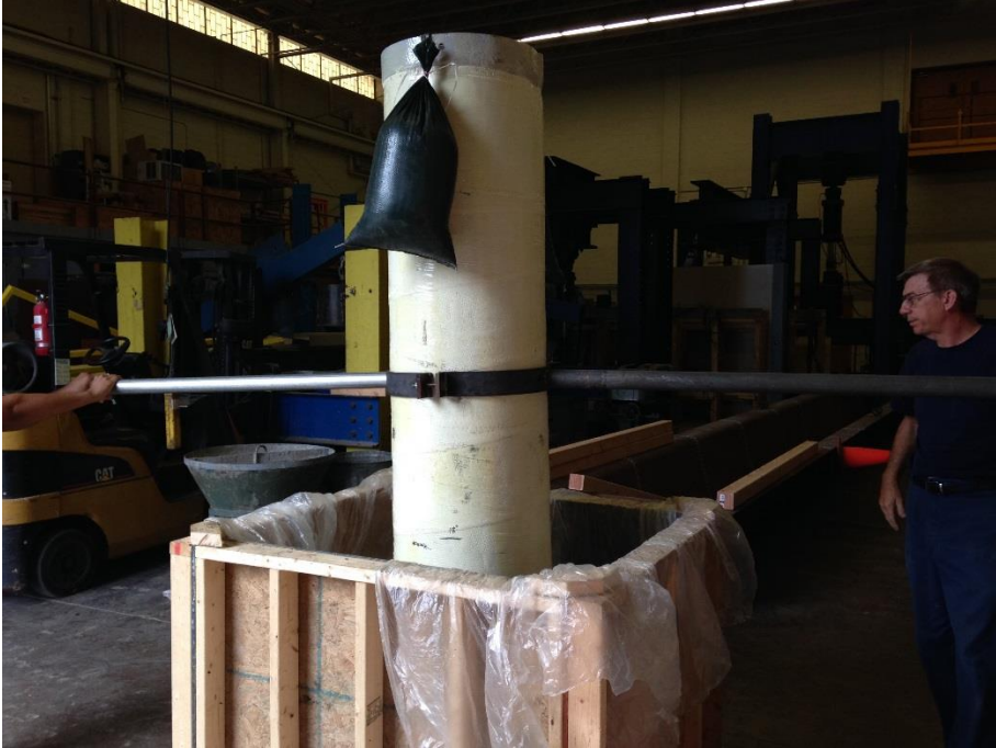
Figure 3-13: Manual application of torque.
