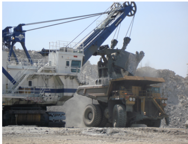
Figure 1.1 Rope shovel and haul truck
