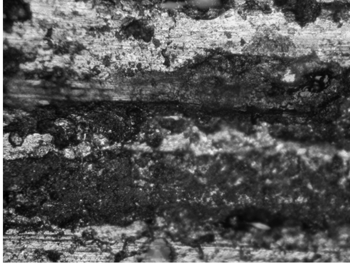
Figure 28 Grooves seen on Stellite 6 surface due to plowing by intermetallic particles
