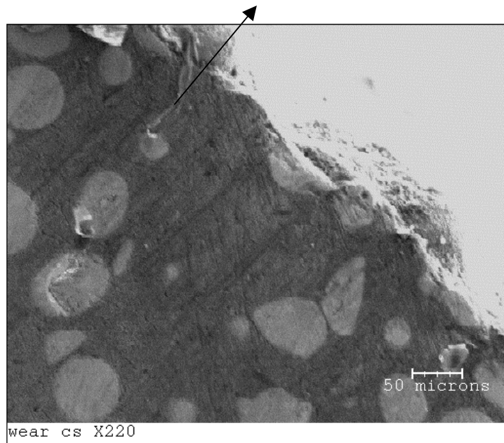
Figure 16 Corrosion crack on the wearing sleeve cross section [1]
