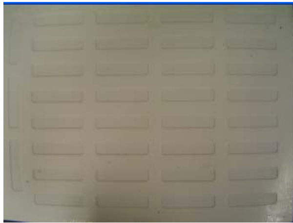
Figure 3 Teflon mold used to cast the samples
