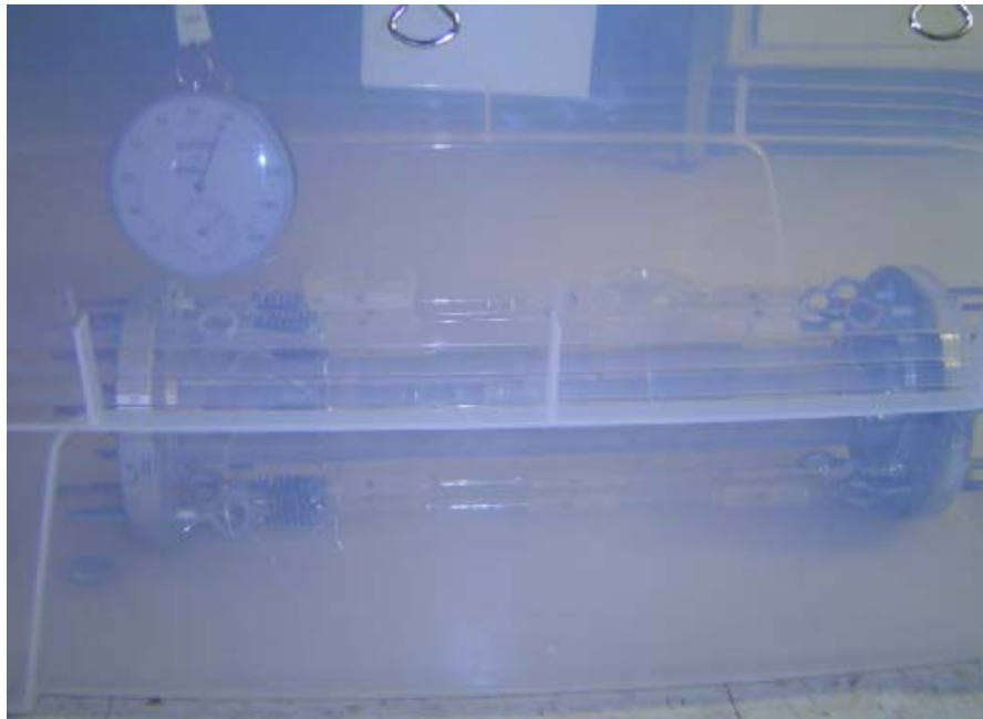
Figure 9 Experimental set up for sorption under stress at 60% RH
