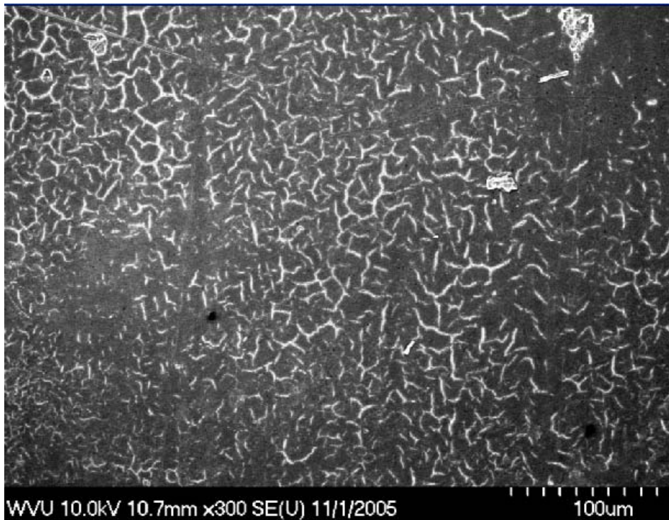
Figure 109 SEM image of 5 wt% clay loaded vinyl ester sample immersed in water and subjected to 30%UTS
