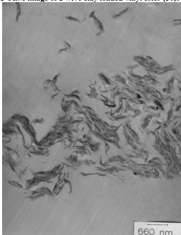
Figure 14 TEM image of 5 wt% clay loaded vinyl ester (30,000x)
