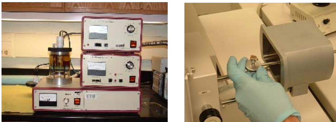
Figure 7 (a) Gold sputter coater (b) Gold coated sample grounded with copper tape
