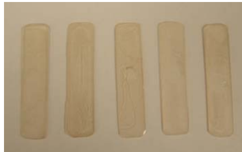
Figure 4 Cured neat vinyl ester samples
