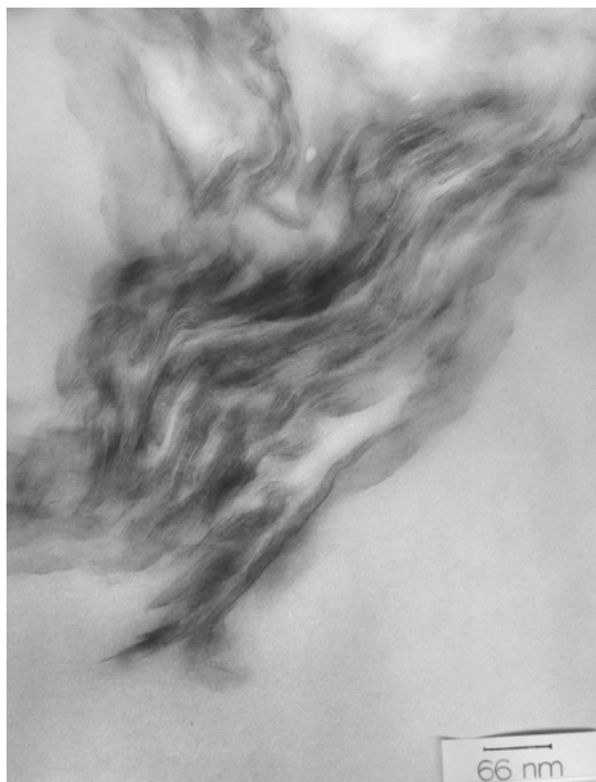
Figure 24 TEM image of 5 wt% clay loaded epoxy (300,000x)
