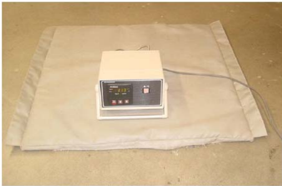
Figure 4.4: Heating blanket with external temperature control box.
