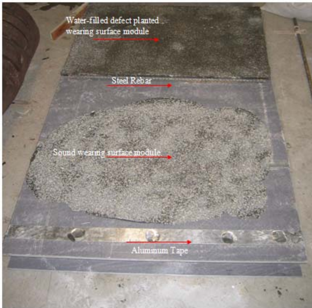
Figure 7.1: The setup of the preliminary GPR test.
