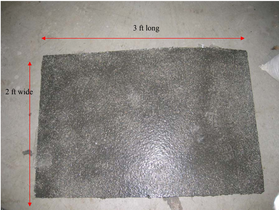
Figure 4.8: Wearing surfaces module of dimensions 36" x 24" x 3/8" (914.4mm x 609.6mm x 9.525mm).
