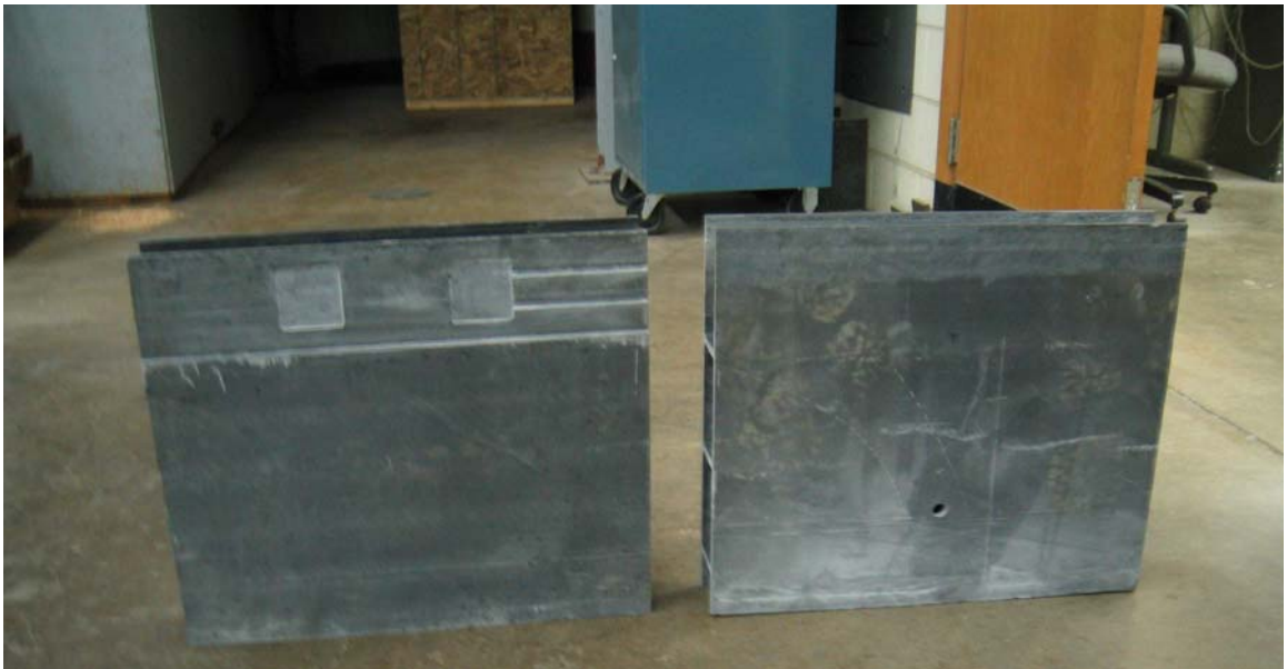
Figure 4.16: The two FRP modules to be joined together.
