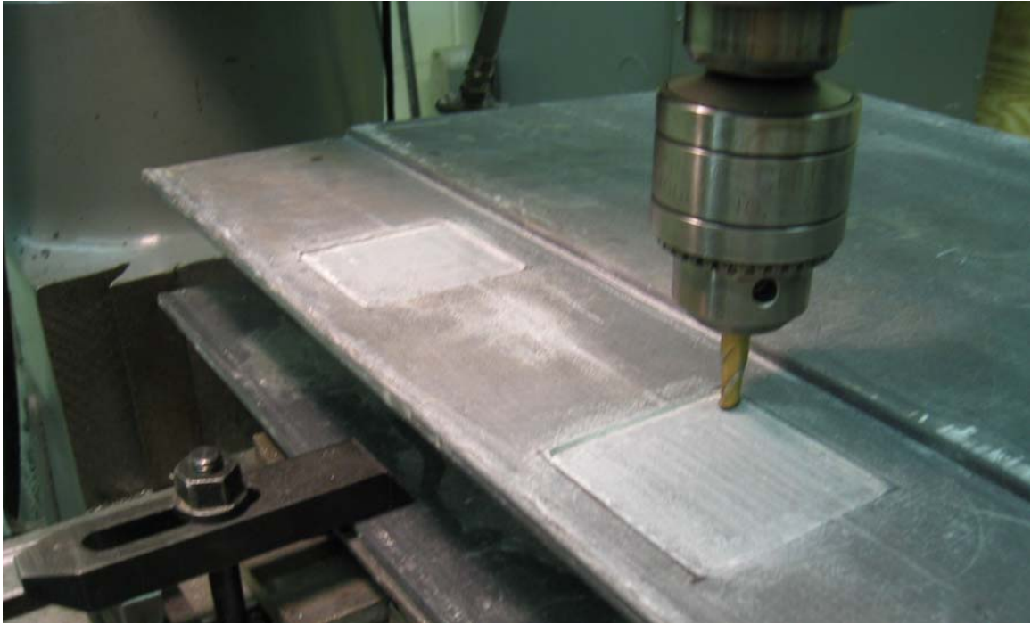
Figure 4.13: The machine drilling out voids to be used as delamination.
