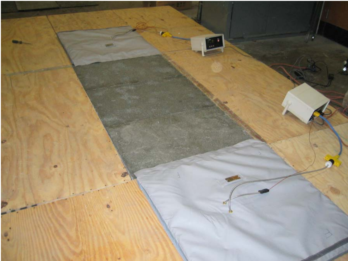
Figure 5.19: The experimental setup for IRT test using heating blanket as active heat source.
