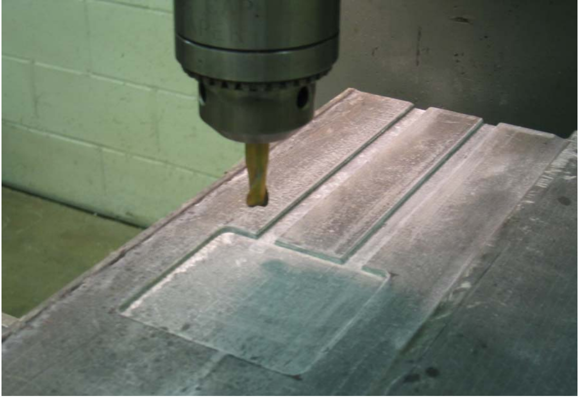
Figure 4.15: Two filling channels were cut out by the machine.
