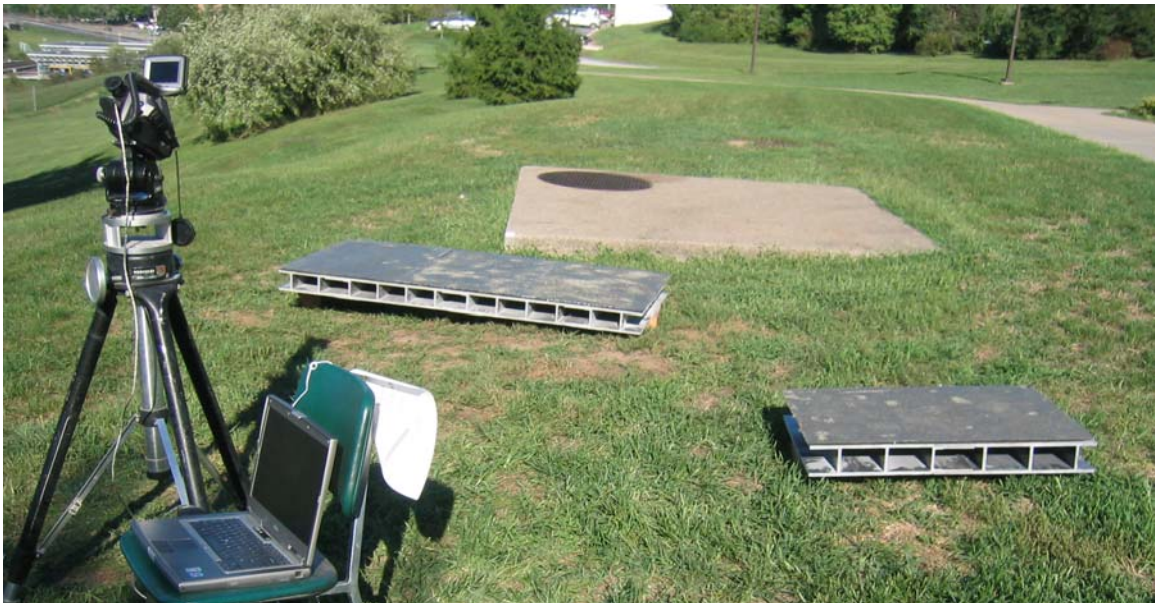
Figure 5.6: The setup of the solar radiation IRT test.
