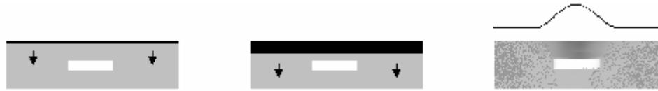
Figure 6.1: Heat flow due to a flash pulse. Initially the pulse causes thin layer of uniform heat on the surface (Left). Heat flows into the sample (Center). When a defect is encountered, the heat is trapped between the defect and the sample surface, giving rise to lateral heat flow above the defect (Shepard et al. 1999).
