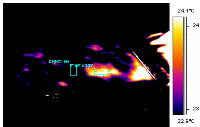
Figure 5.25: Results of IRT on water-filled defects using heating blanket as active heat source.
