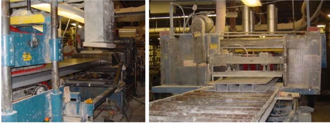
Figure 4.7: Photographs showing manufacturing of FRP bridge deck in a factory using Pultrusion process.
