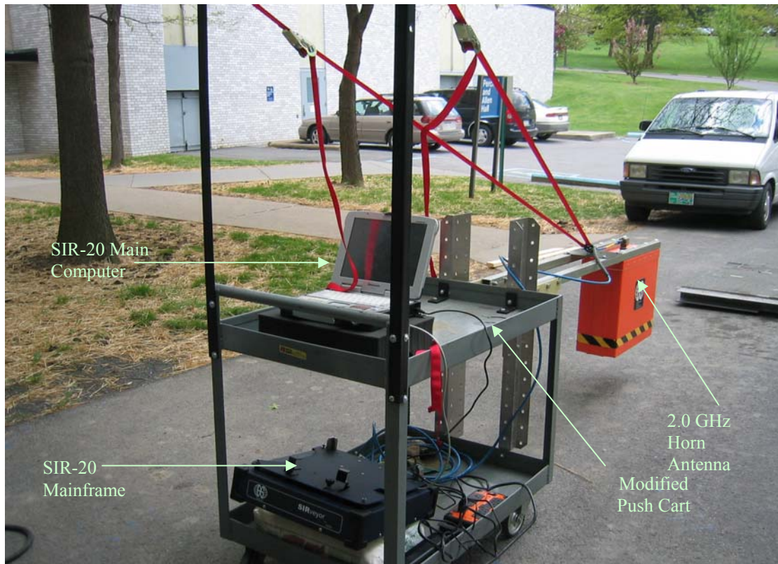
Figure 4.1(a): GPR system with 2.0 GHz horn antenna on the modified push-cart.
