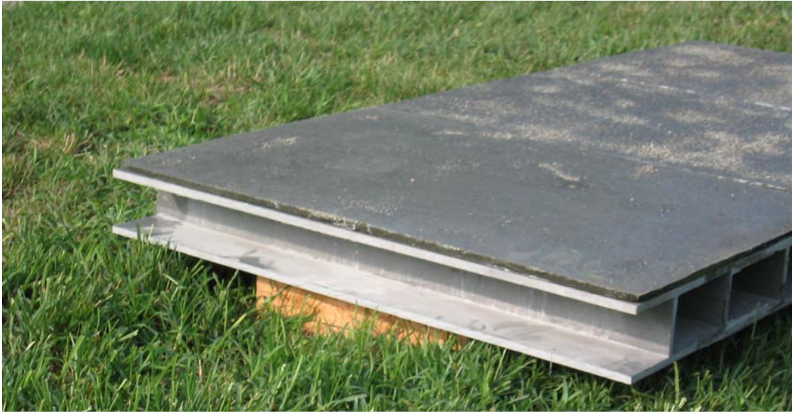
Figure 5.5: The bridge deck module with wearing surfaces.
