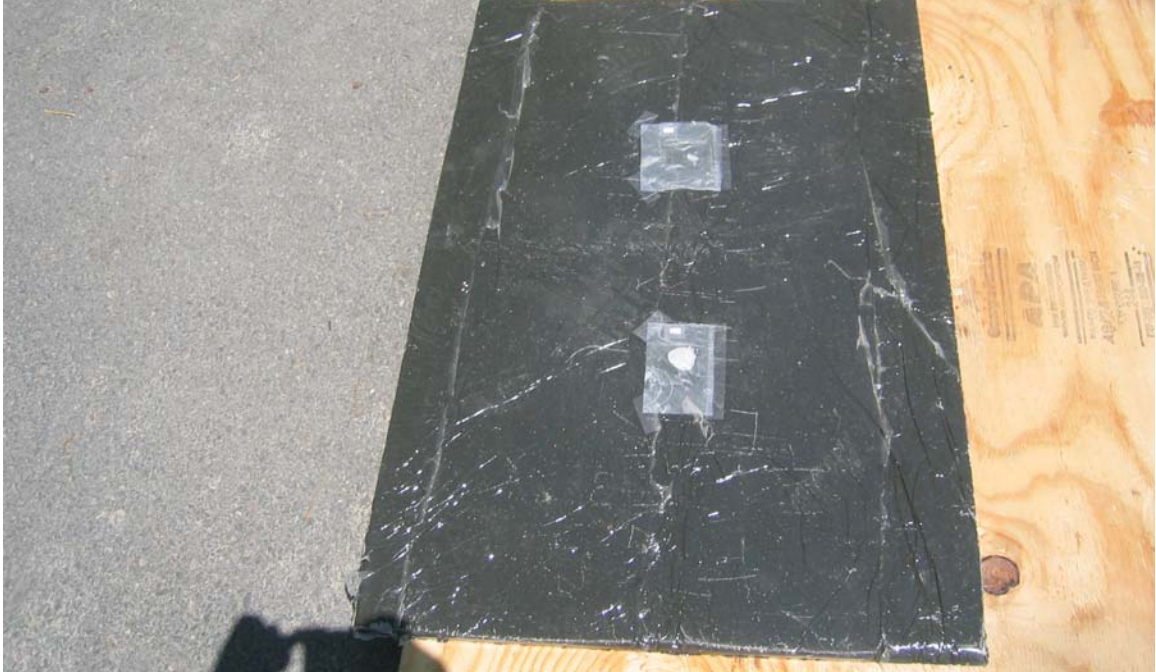
Figure 4.12: Bottom side of a wearing surface with two water-filled simulated debonds attached.
