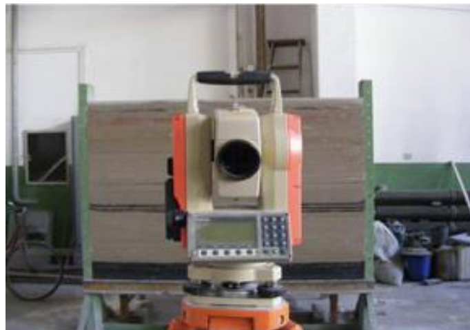
Figure 1-2 Electronic Total Station for Survey Data Acquisition
