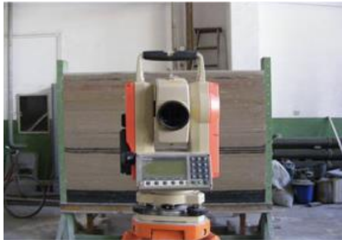
Figure 2-3 Electronic Total Station for Survey Data Acquisition
