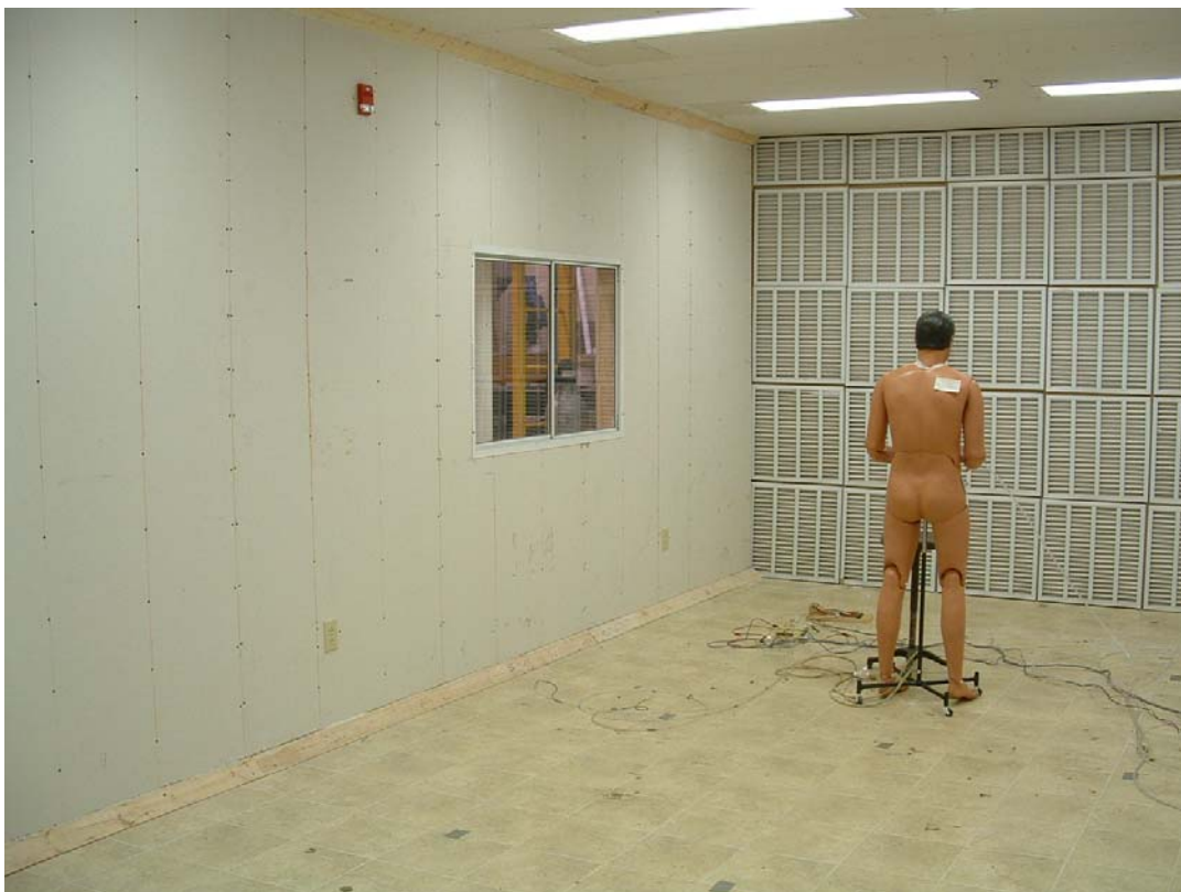
Figure Appendix 1.1 Wind tunnel with mannequin.
