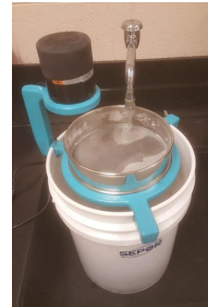
Sepor Sieve Shaker 4) 20 - 30 minutes of wet sieving
