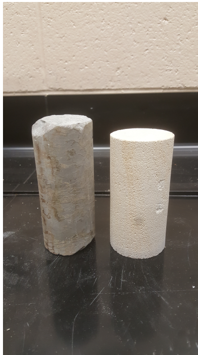
Figure 3.1: Limestone (L) and Chalk (R) Cores
