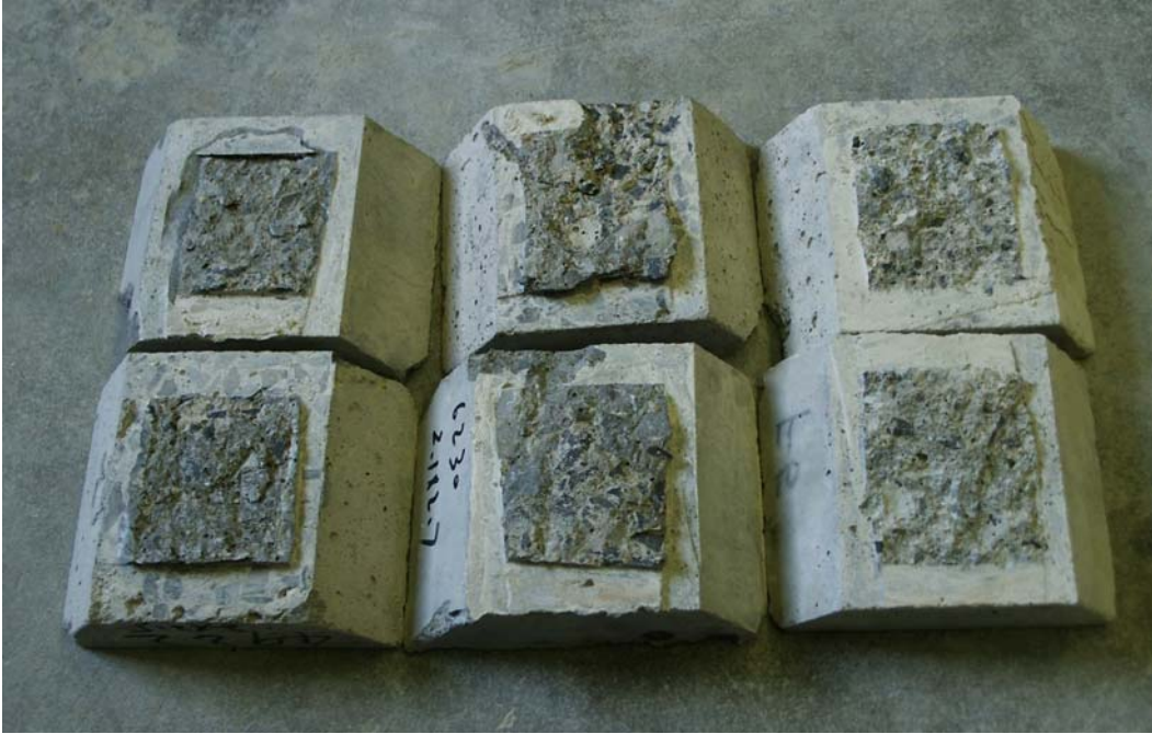
(c) Failure of Surface Preparation CSP #8
