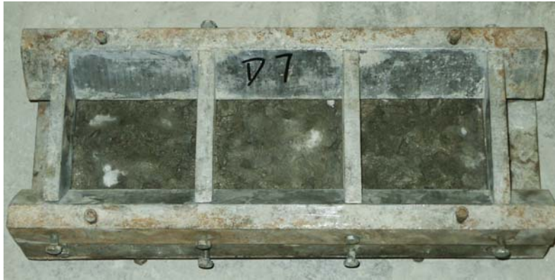
Fig. 5.5–Install the substrates back to molds
