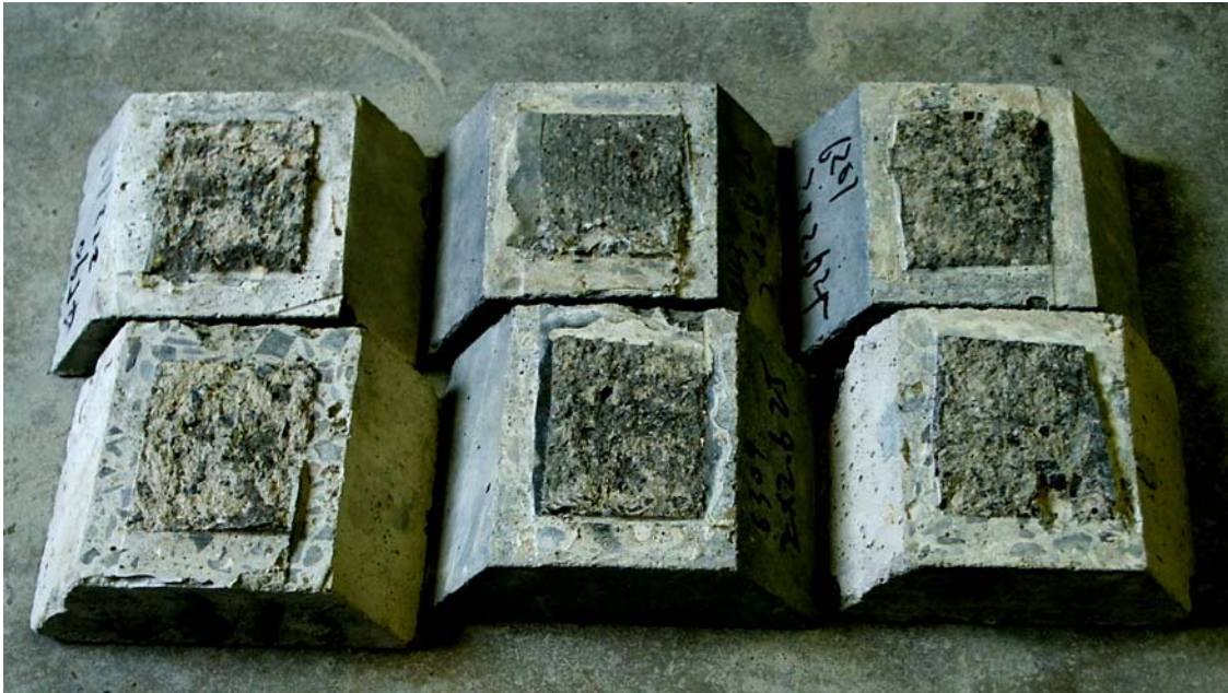
(a) Failure of Surface Preparation CSP #5
