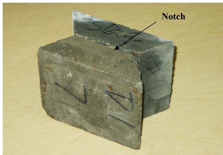
Fig. 5.7–Bi-Layer specimen with notches all around
