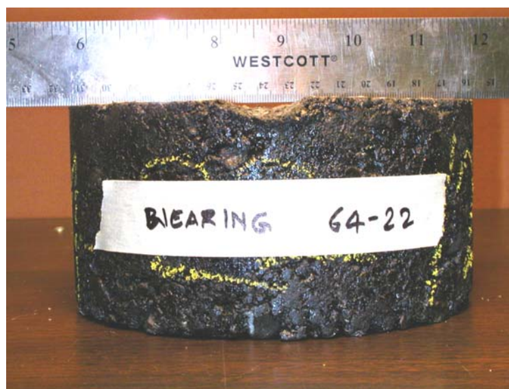
Figure 4.1 Sample after APA testing, 12.5 mm specimen, field gradation and PG 64-22 binder
