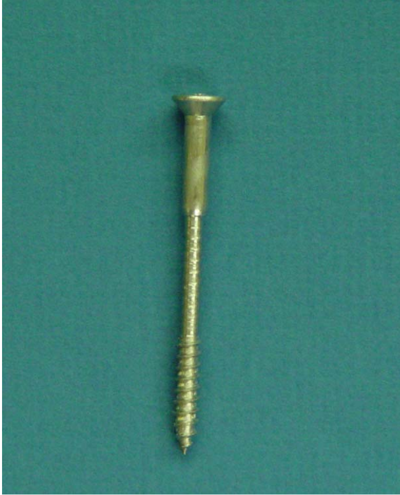
Figure 2.6. - Screws used for screw withdrawal testing.
