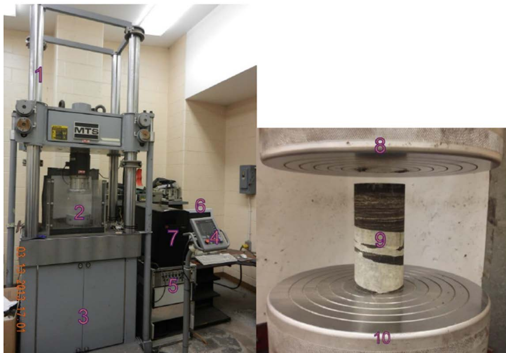
Figure 6.7 MTS servo controlled compression testing machine and its component 1) Machine Load (2) Glass Shield (3) Hydraulic Actuator (4) Manual Control System (5) Strain Gauge Control Panel (6) Computer (7) MTS Data Acquisition System (8) Upper steel platen with circular grooves (9) Specimen (10) Lower steel platen with circular grooves
