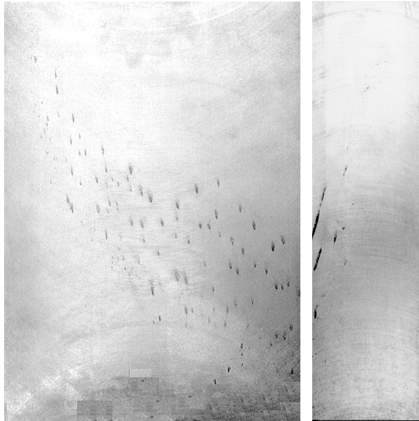
Figure 3-1: Cut-up surfaces showing freckles decorating pool profiles.
