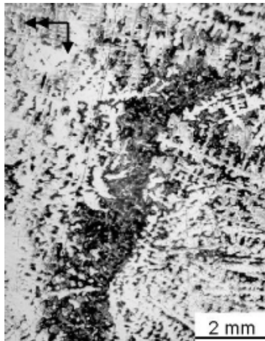
Figure 3-12: Longitudinal section of freckles in HV8853 showing the irregularities of dendrites and downward freckle flow. (Gravity force points downwards and ingot grows to the left)
