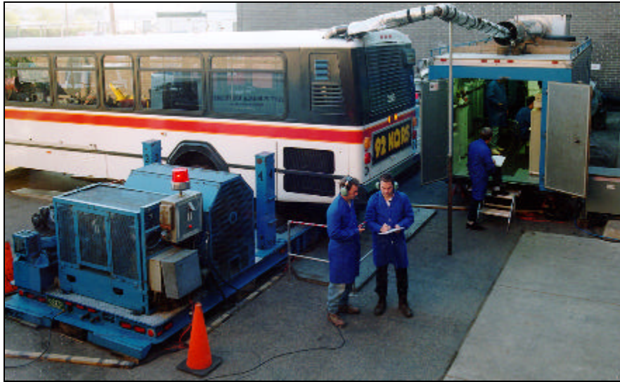
Figure 1.3 Transit bus being tested on the WVU THDVETL with flywheels and power absorber in foreground and dilution tunnel atop analyzer trailer at the rear of the bus.
