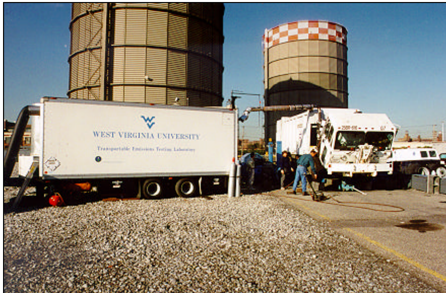
Figure 1.2 Refuse truck being tested on the WVU THDVETL showing exhaust routed into dilution tunnel inside the analyzer trailer.
