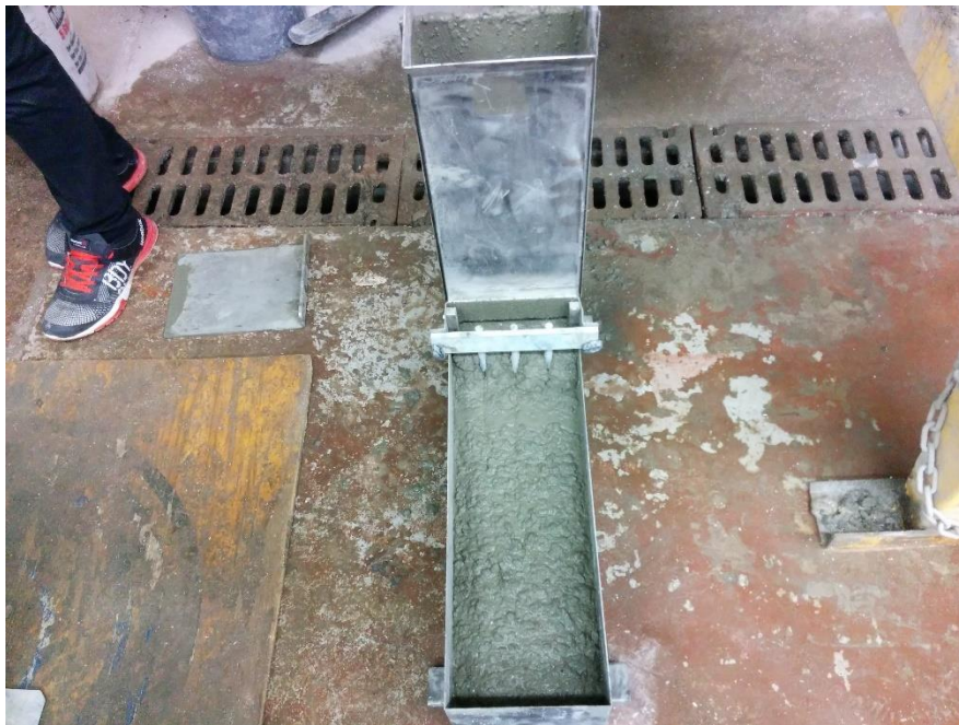
Figure 3-8 – L-Box Apparatus after Concrete Flow
