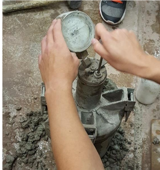
Figure 3-5 – Determining the Air Content of 50% Slag Batch using Type B Air Content Apparatus
