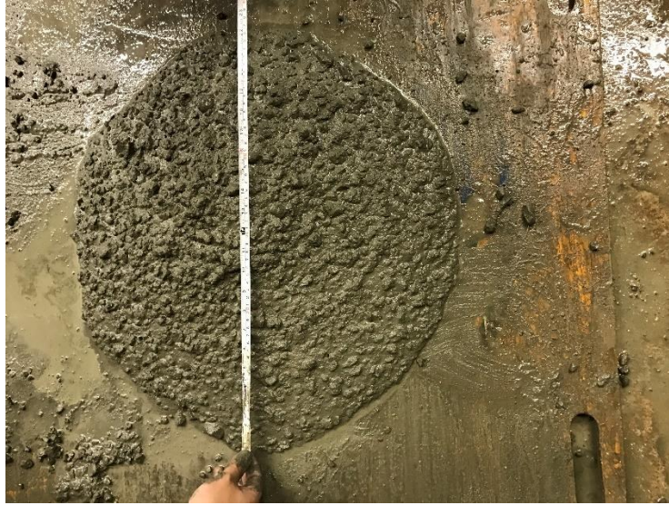
Figure 3-6 – Slump Flow Measurement ( d_1 )
