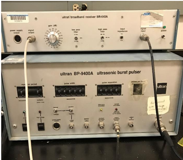
Figure 3-14 – Pulse Generator and Broadband Receiver Amplifier
