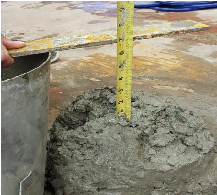
Figure 3-3 – Slump Test Result for 50% Slag Batch
