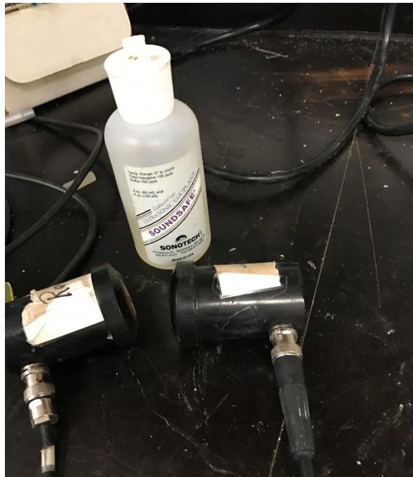
Figure 3-16 – Pulsar Transmitting Transducer (Right) and Receiving Transducer (Left) and Coupling Agent
