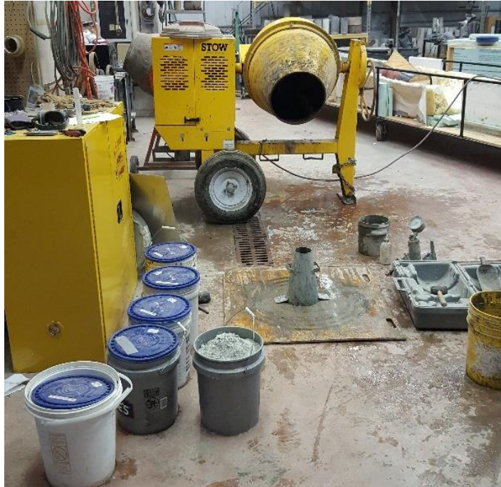
Figure 3-1 – Drum Mixer, Materials, and Slump Test Setup – 50% Slag Casting
