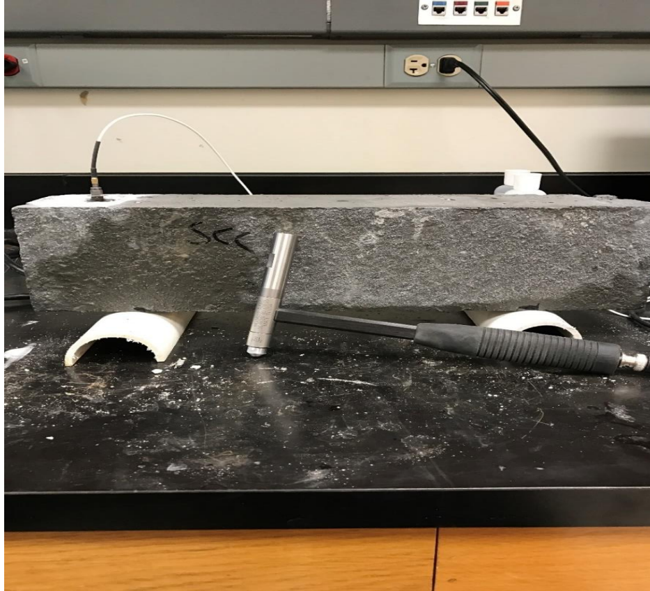
Figure 3-20 – Impact Hammer, Accelerometer, and Specimen used in Study
