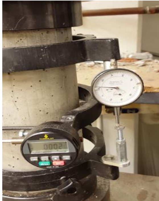
Figure 3-10 – Static Modulus Apparatus Consisting of Compressometer Gage (Dial Gage) and Extensometer Gage (Digital Gage)
