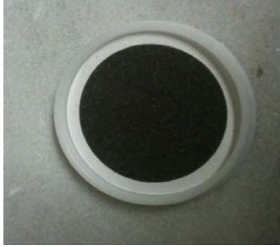
Figure 5-29 Gravimetric filter sample after 9 hours of PM sampling during the idle operation
