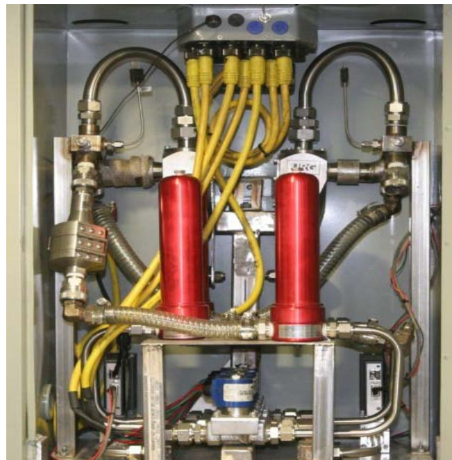
Figure 3-6 CFR 40 Part 1065 compliant PM sampling system on-board the transportable laboratory container
