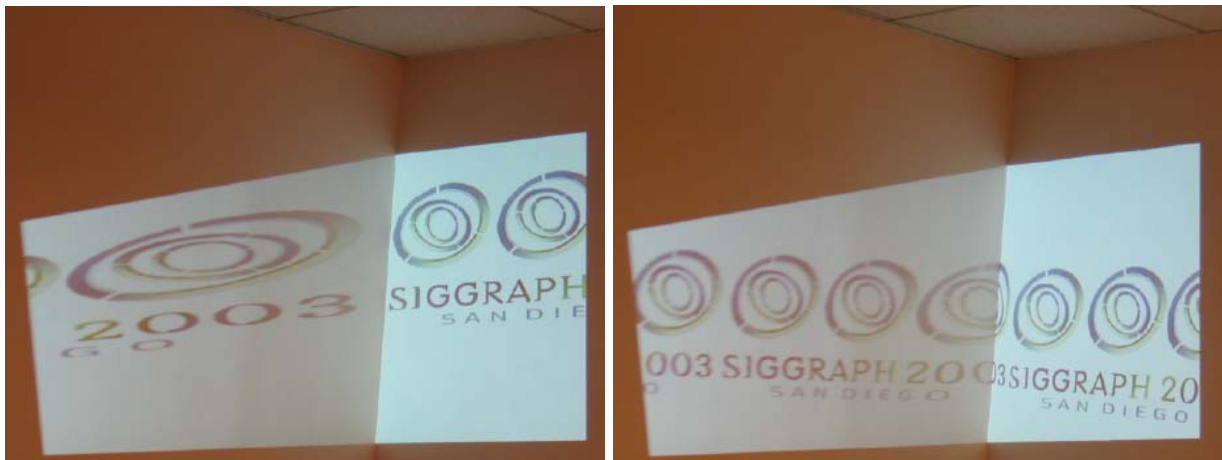
Figure 11 The use of image warping in correcting distortions produced by projecting images from an LED source onto a wall; left: skew image produced by uncorrected projection; right: same projection with correction algorithm described by Raskar et al. [46, p. 811].
