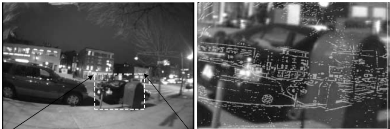
Figure 9 Peli et al. augmented-view concept; left: full view of a street scene taken at night, where the white rectangle represents the size of the field of the display (e.g. that of an RP patient or other minimal view application); right: edge-contour image of the same scene (on the left) superimposed on the natural view (shown here as the car and mail box in the edge-contour image) [7, p. 297].
