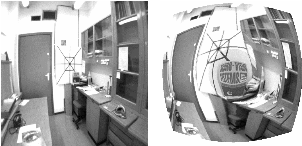
Figure 8 Amerijckx et al. technique for central vision magnification with a remapping algorithm similar to that of Juday-Loshin but using two CCD cameras; left: original image; right: warped image, with highly enlarged central image, yet with also a highly distorted overall image [2, p. 381].
