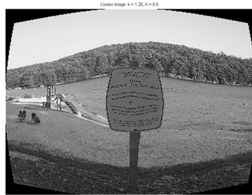
Figure 34 Demonstration for applying the convex or “fish-eye” technique to a sample image (image 3 “text,” from image set 1) using different k (remapping) and K (proportionality) parameters; the first three images involve varying K (0.4, 0.7, 1.0) at the fixed, default k (1.15), and the last three involve varying k (1.10, 1.15, 1.20) at the fixed default K (0.5); note the compromise between increased convexity ( k ) and increased image distortion, as well the decreased resolution due to resizing reduced-size images for various K factors.
