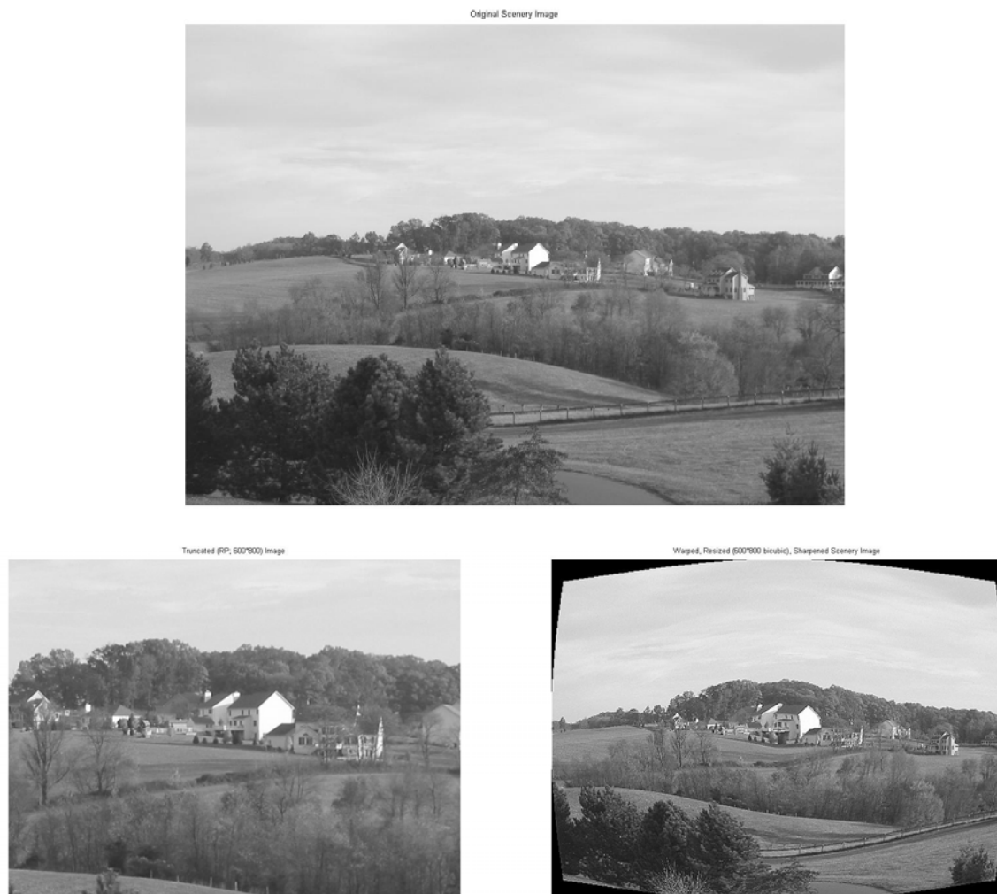
Figure 17 Matlab ® code demonstration for warping a scenery image using the convex projection method; top: base image (grayscale used for simplification); bottom left: truncated (or viewable) image, included for comparison; bottom right: warped image, resized to 600*800 pixels for standardization, with bicubic interpolation method used for higher calculation accuracy, and filtering applied to increase image sharpness.
