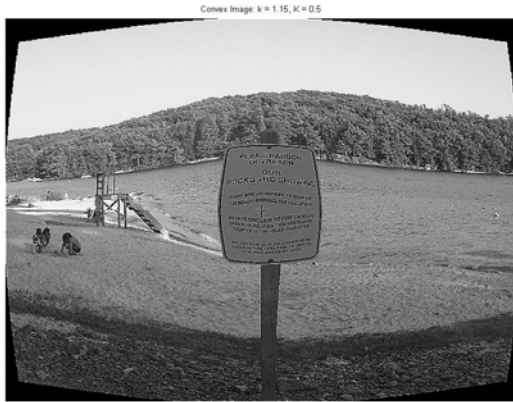
Figure 34 Demonstration for applying the convex or “fish-eye” technique to a sample image (image 3 “text,” from image set 1) using different k (remapping) and K (proportionality) parameters; the first three images involve varying K (0.4, 0.7, 1.0) at the fixed, default k (1.15), and the last three involve varying k (1.10, 1.15, 1.20) at the fixed default K (0.5); note the compromise between increased convexity ( k ) and increased image distortion, as well the decreased resolution due to resizing reduced-size images for various K factors.
