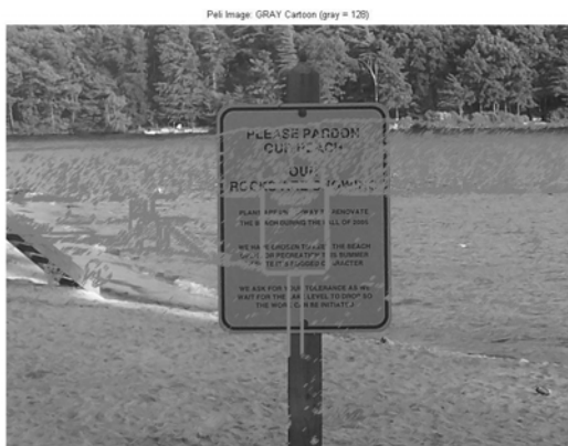
Figure 29 Demonstration for applying the “Peli” superimposition technique to a sample image (image 3 “text,” from image set 1) using different gray shades; top-left: black cartoon (luminance: 0); top-right: white cartoon (luminance: 255); bottom-left: gray cartoon (luminance: 128); bottom-right: mean cartoon (luminance: 133); note how in all cases, the sign is almost completely dominated by the cartoon.
