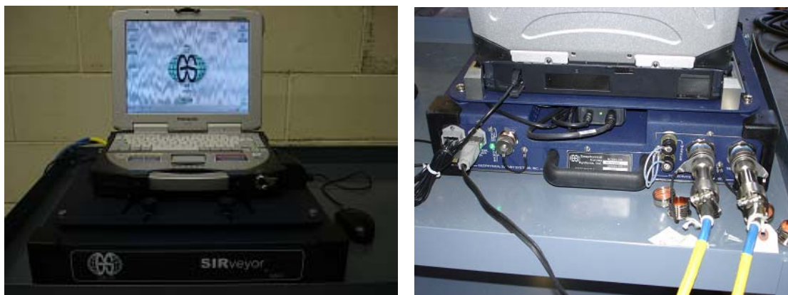
Figure 3-2 Data acquisition system (laptop computer and main frame)
