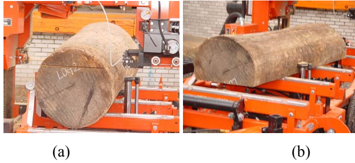
Figure 5-19 Sawing of Log 2 using a portable saw mill
