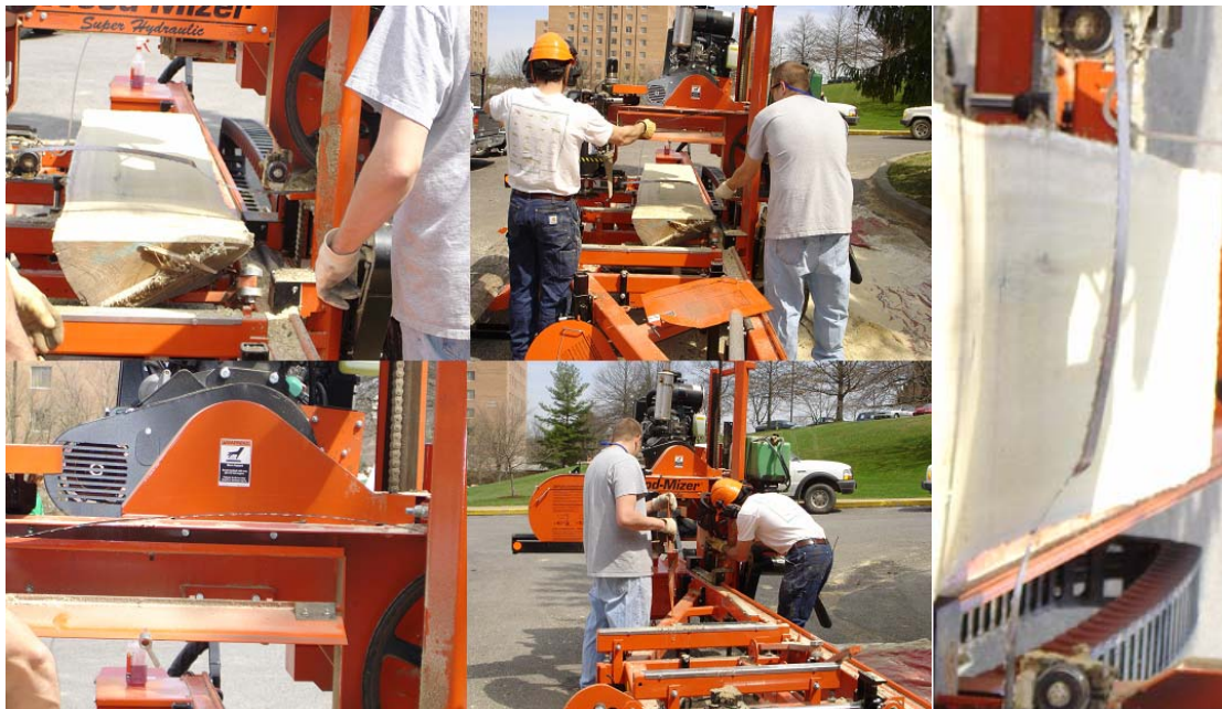
Figure 5-54 Picture showing the problems faced after the saw blade hit the small metal piece and got bent, and subsequent replacement of the blade
