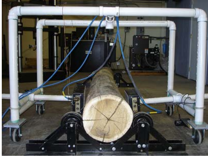
Figure 5-82 Two antenna on the side in T1R1 and T2R2 mode
