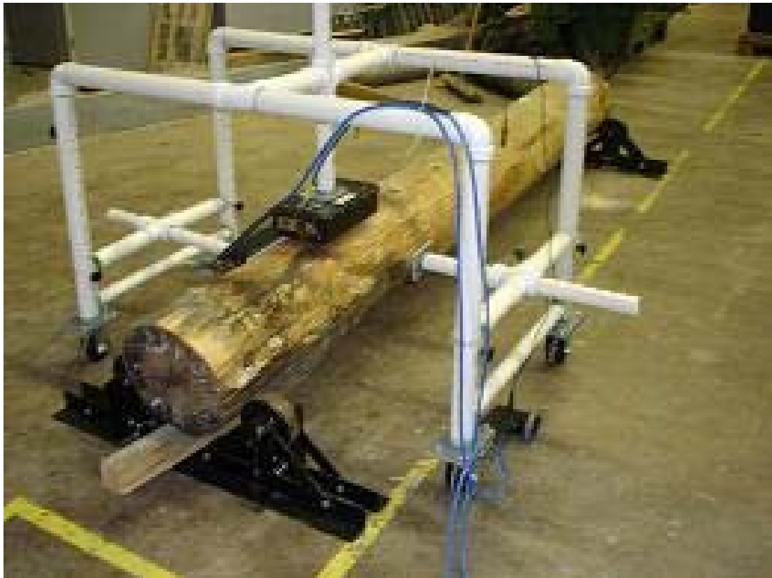
Figure 5-1 Antenna configuration for Log 1
