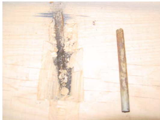
Figure 5-23 Inserted metal rod defect
