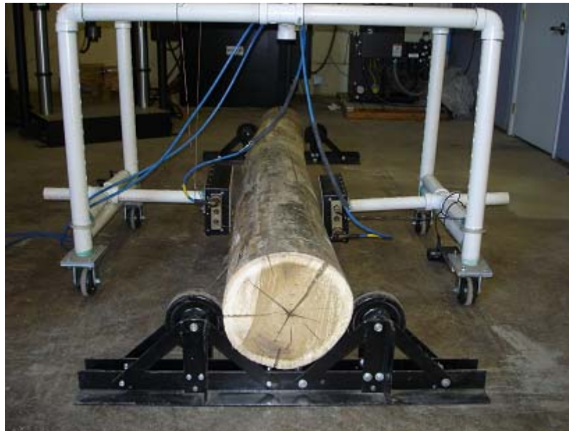
Figure 5-85 Two antennas on the side in T1R2 and T2R1 mode
