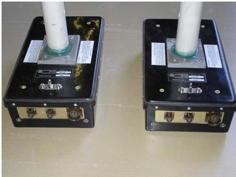
Figure 3-3 Two 900 MHz antennas
