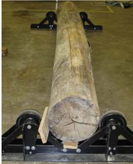
Figure 4-2 Picture showing wooden pieces under the small end of the Log 4 to raise the level
