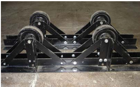
Figure 3-6 Rollers for supporting and rotating logs
