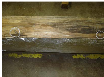
Figure 4-5 Aluminum foil at the opposite face of the log
