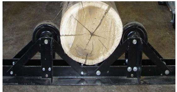
Figure 3-6 Rollers for supporting and rotating logs
