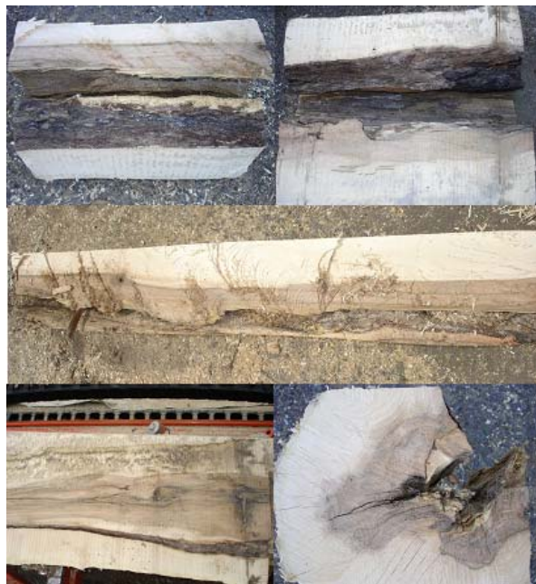
Figure 5-34 Pictures showing the extent of decay (rot) in Log 3
