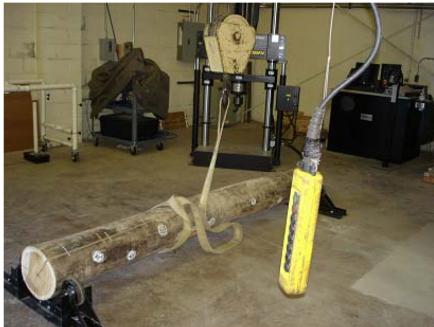
Figure 3-8 Showing the crane and the control switches for lifting the logs
