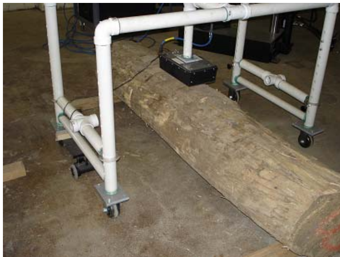
Figure 5-59 Antenna configuration for Log 6
