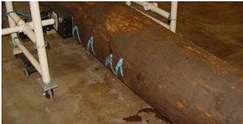
Figure 5-46 Log 5 and the antenna configuration used for collecting GPR data
