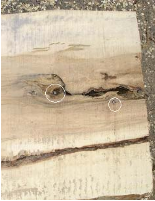
Figure 5-35 Location of metal nails
