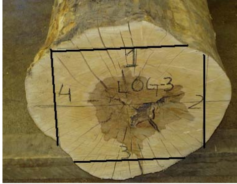
Figure 4-1 Lines marked on Log 3 for GPR scanning and sawing purpose
