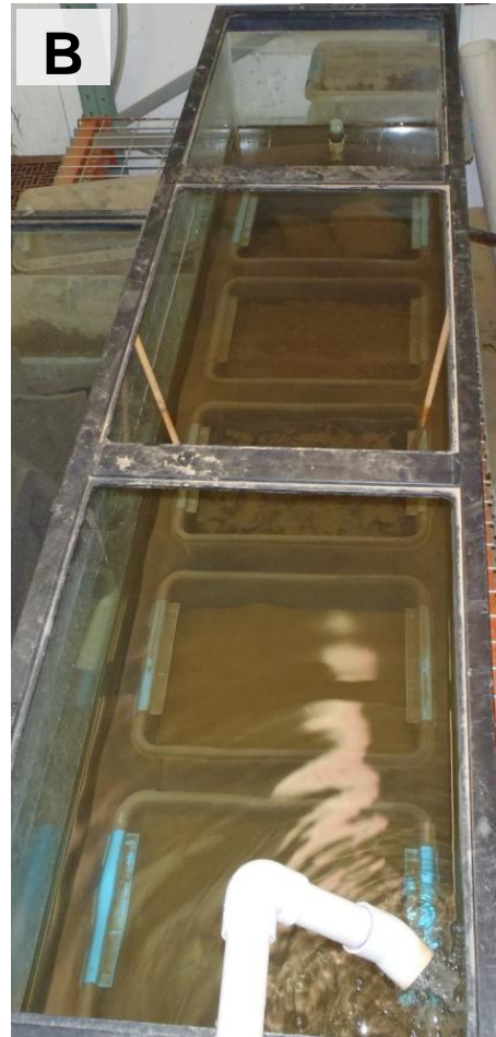
Figure 2.2. Photograph A shows the aquarium setup with one substrate bin removed to show fish friendly foam in place. Photograph B is the aquarium setup with substrate bins and fish friendly foam. Note the leaf pack substrate bin is being held in place by two wooden dowels.
