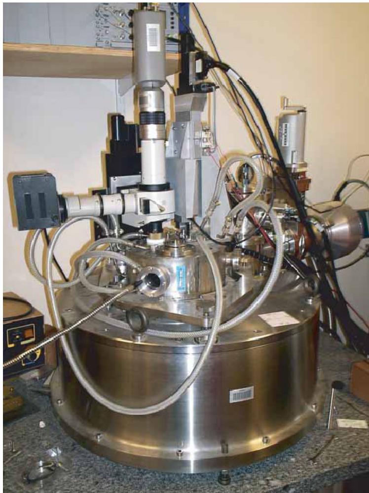
Figure 9: Instrumented micro-indentation equipment for experiments up to 1000°C [38].
