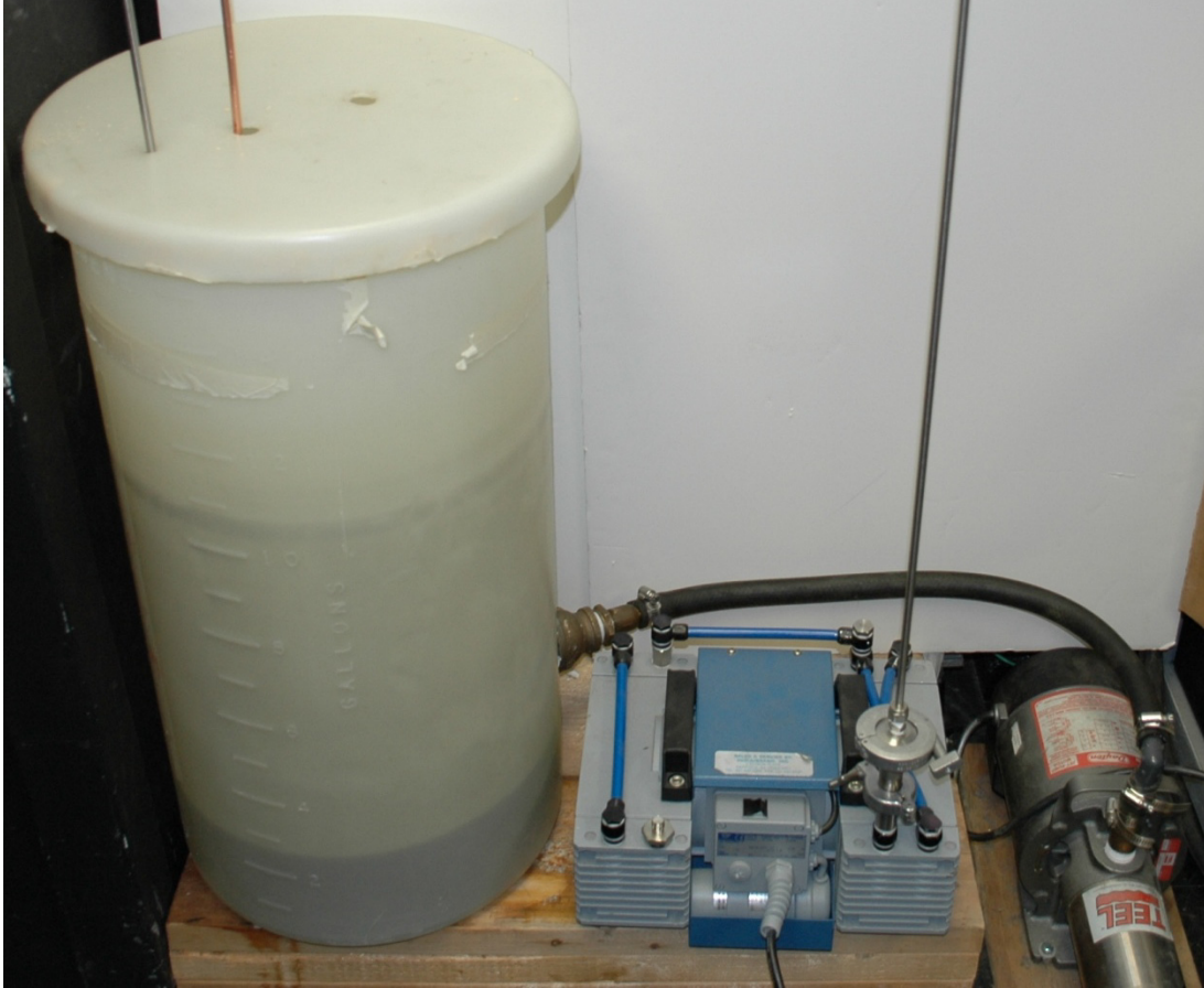
Figure 18: Controlled environment high temperature indentation system, external water pumps and cooling tank.
