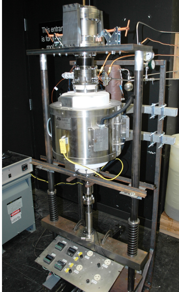
Figure 19: Controlled environment high temperature indentation system; overview.
