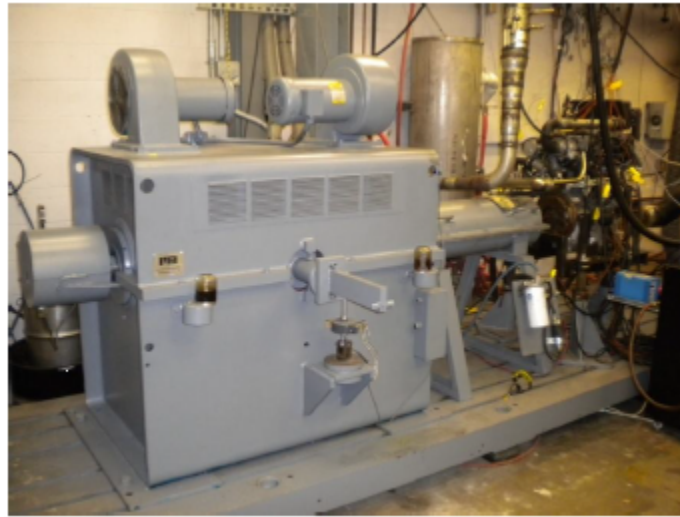
Figure 18: Medsker Electric Inc. alternate current dynamometer
