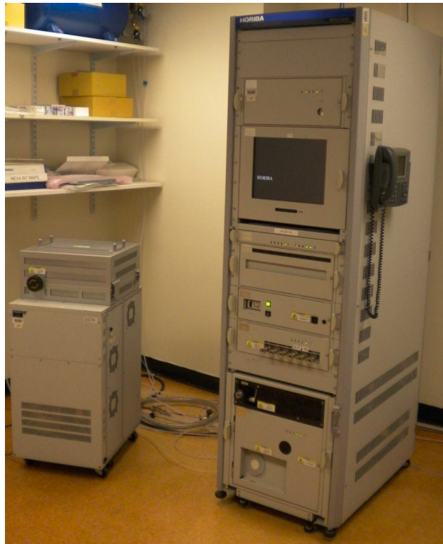
Figure 13: Horiba Automotive Emission Analyzer System MEXA 7200D
