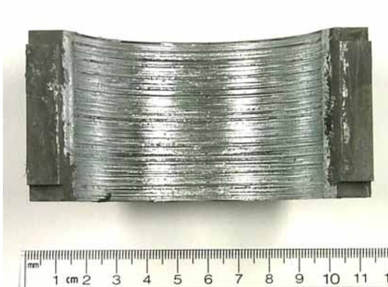
Figure 4-18: Stellite#6 Bushing (Static) Following Wear Test (Data Shown above) [reprinted with permission from The International Lead Zinc Research Organization, Ref. 39]
