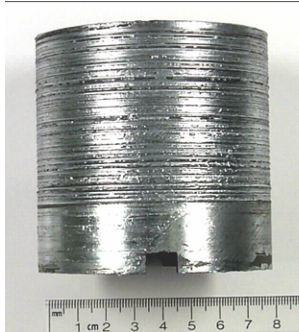
Figure 4-17: Stellite#6 Bearing (Rotating) Sleeve Following Wear Test (Data Shown above) [reprinted with permission from The International Lead Zinc Research Organization, Ref. 39]
