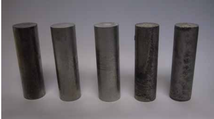
Figure 5-4: 316L stainless corrosion samples after pickling in a dilute (15%) HCl solution
