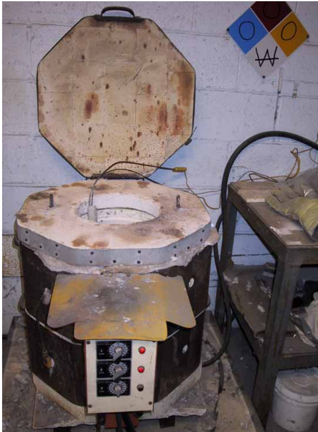
Figure 5-1: Electric-resistance-heated kiln furnace with silicon carbide crucible
