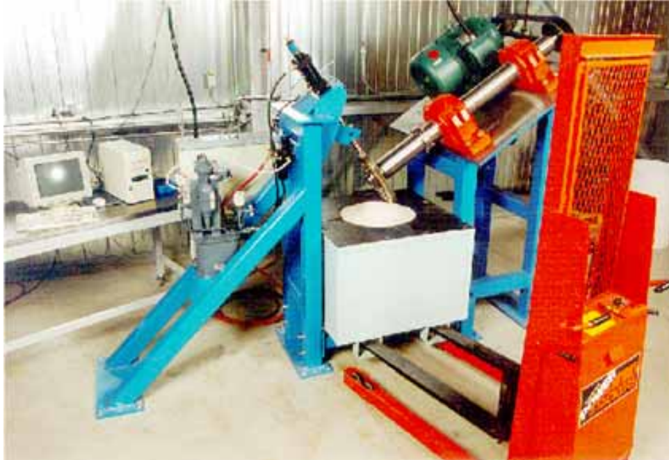
Figure 4-13: Full-Scale Bearing Wear Tester at Teck Cominco Product Technology Centre [reprinted with permission from The International Lead Zinc Research Organization, Ref. 39]
