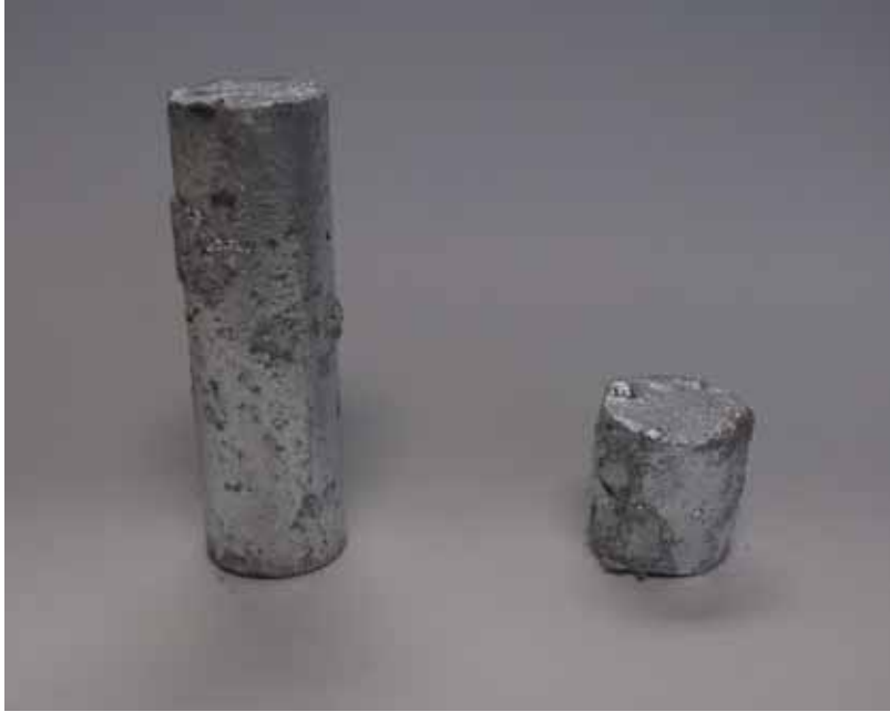
Figure 5-3: 316L stainless corrosion sample and microscopy sample after immersion in zinc
