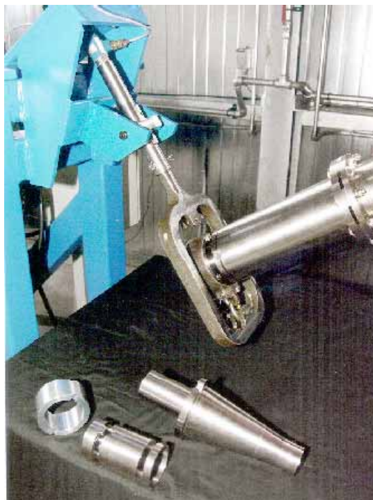
Figure 4-14: Bearing Test Sample Attachment Apparatus [reprinted with permission from The International Lead Zinc Research Organization, Ref. 39]
