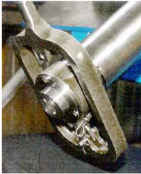
Figure 4-15: Assembled Bearing Sample in Test Rig [reprinted with permission from The International Lead Zinc Research Organization, Ref. 39]
