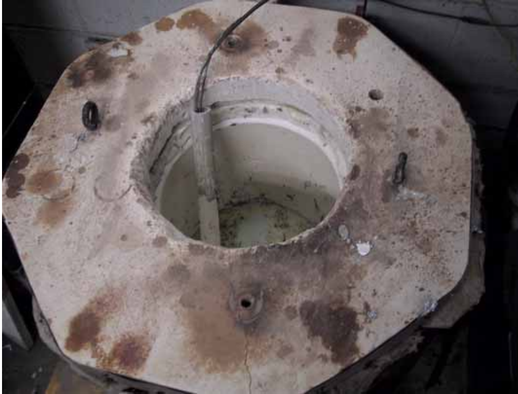
Figure 5-2: Silicon carbide crucible containing molten zinc bath
