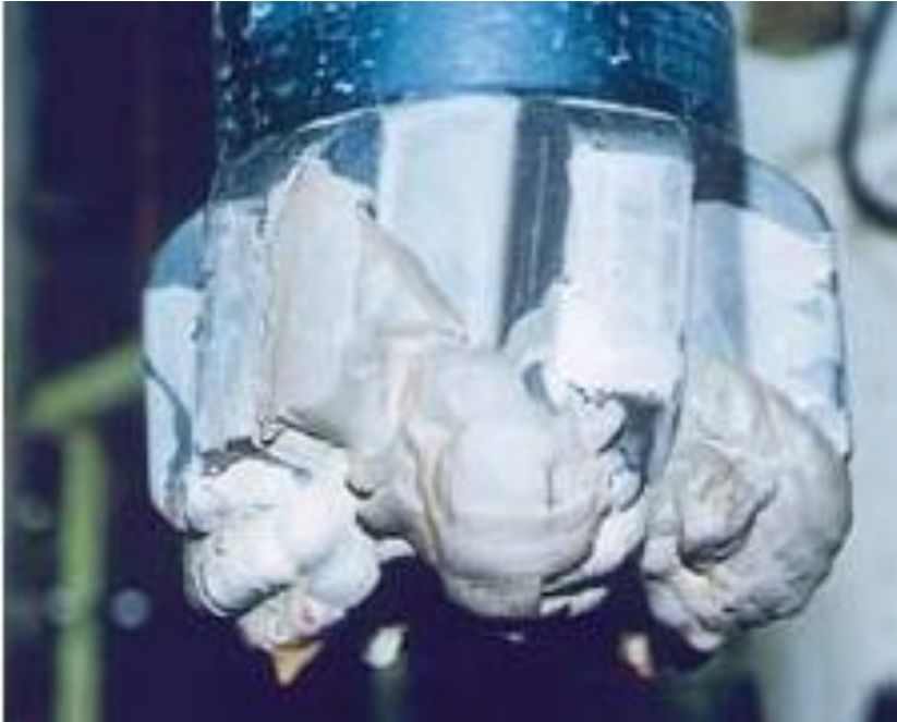
Figure 1.3: Bit balling reduces penetration rate ( Oil and Gas Journal , www.ogi.com )
