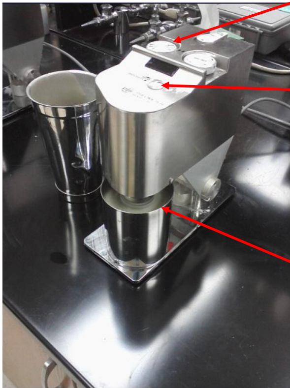
Figure 3.9: Rheometer for PV measurement demonstration
