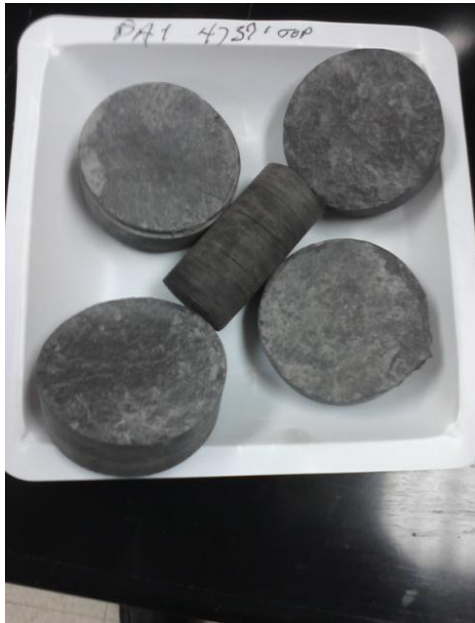
Figure 3.13: Uncrushed Marcellus Shale samples from WV#6 well in West Virginia. 4737 ft (Courtesy of US DOE)
