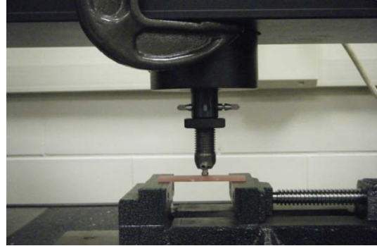
Figure 7. Load centered in specimen center
