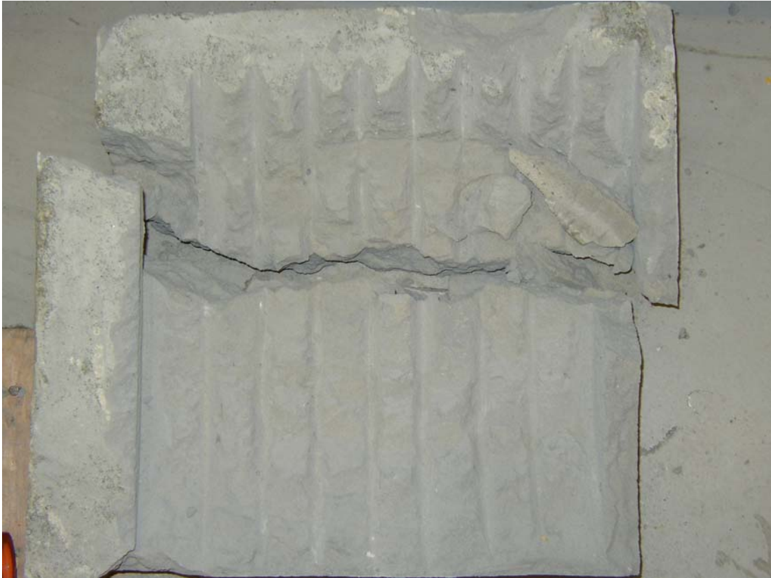
Figure 3.13 . Multiple Cutting in the specimen block (bit B)
