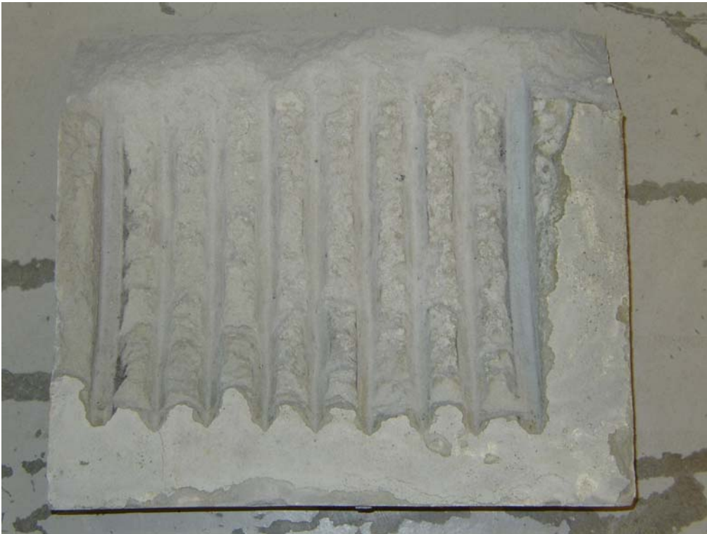
Figure 3.12 . Multiple Cutting in the specimen block (Bit C)
