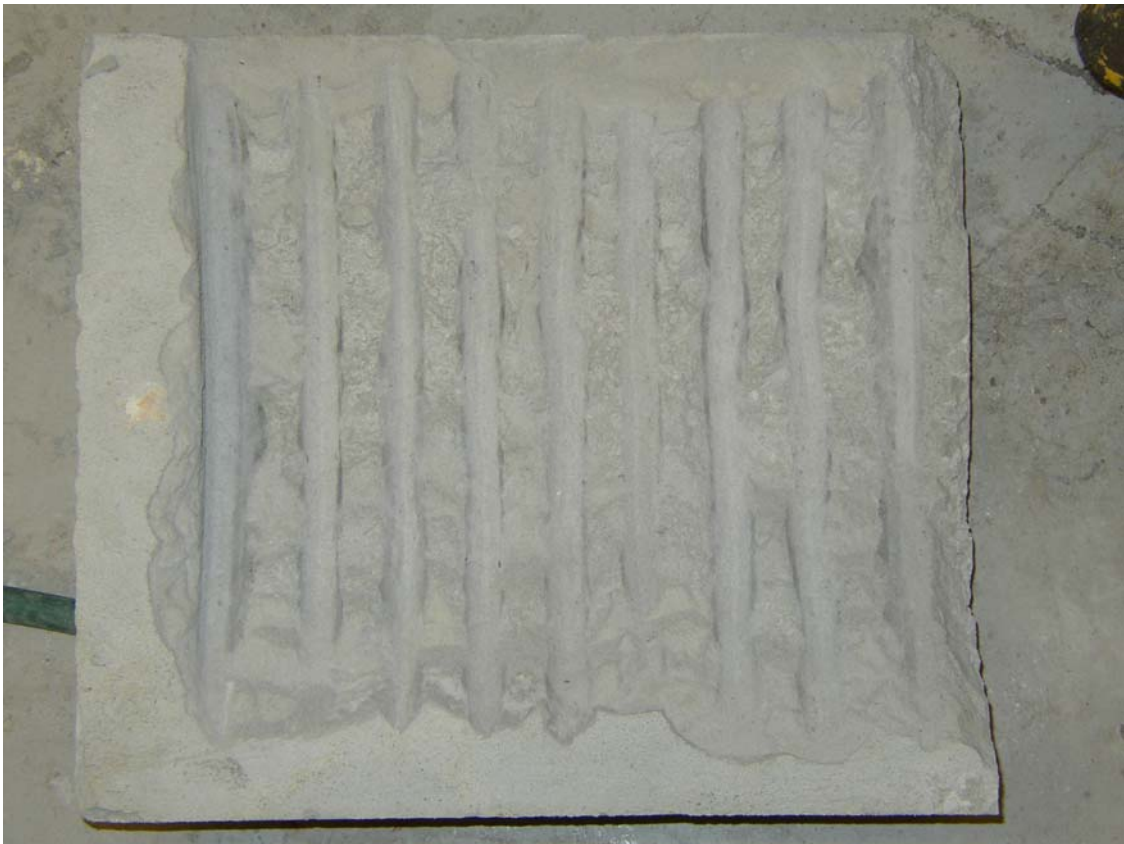
Figure 3.14 . Multiple Cutting in the specimen block (Big A)
