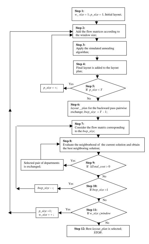
Figure 4.15: SA COMBO algorithm
