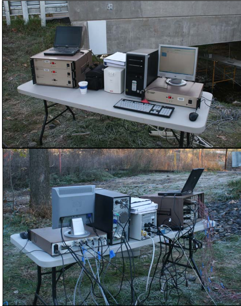
Figure 3.11 Data Acquisition Setup
