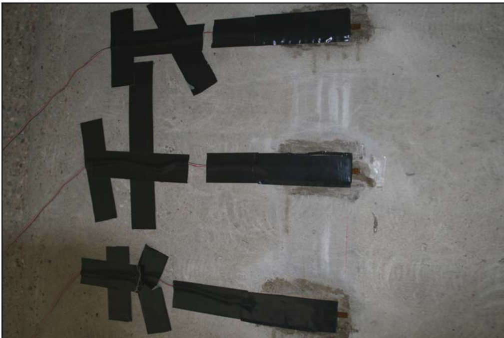
Figure 3.5 Concrete Gage with Barrier E Protective Coating
