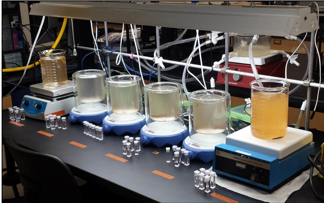
Figure 4-7. Photograph of the filtering experiment for Fe analysis. Vessels are numbered 1 through 6 from left to right. Vessels 1 and 6 are beakers, and vessels 2 through 5 are jacketed reaction vessels.
