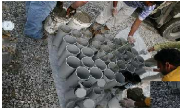
Preparation of Cylindrical Specimens
