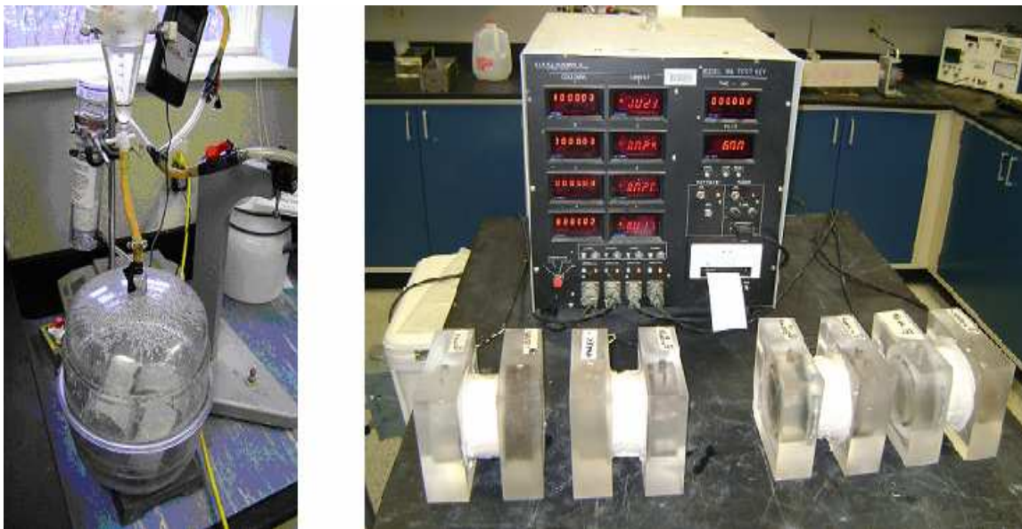
Figure 4-10 Conditioning and testing samples for RCPT
