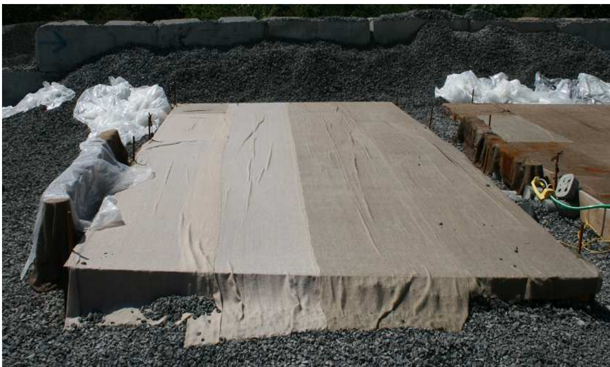
Figure 3-5 Slabs and match-cured specimens
