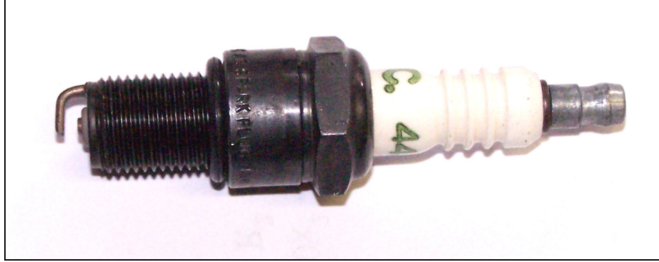
Fig. 24 Spark plug use in ignition experiments
