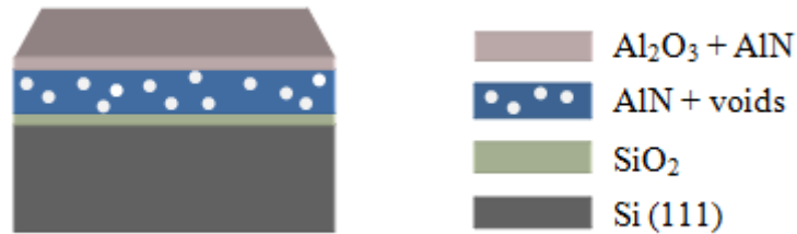
Figure 3.11. Three layer model of a reactively sputtered AlN film on silicon. After Mahmood et al. [Mahmood, 2003].
