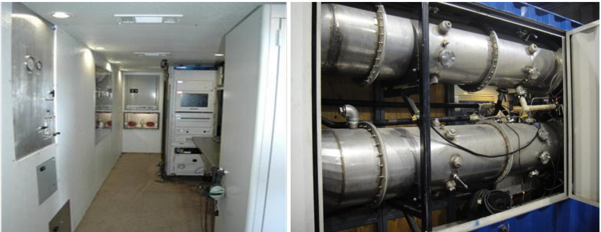
Figure 3.9 MEXA 7200D analytical bench and the full scale CVS dilution system onboard WVU CAFEE's TEMS
