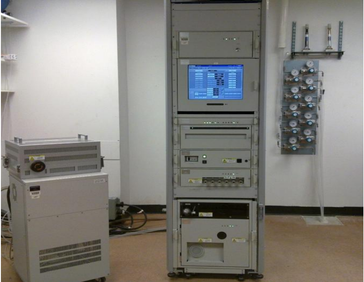
Figure 3.8 MEXA 7200D analytical bench at WVU CAFEE's EERL facility
