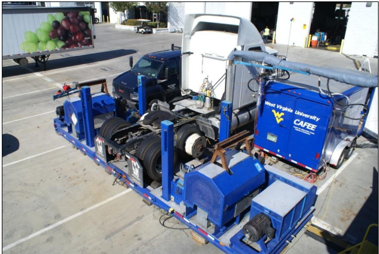
Figure 3.5 View of the Diesel with DOC-DPF-SCR vehicle being tested on WVU CAFE's transportable heavy-duty chassis dynamometer at the test facility
