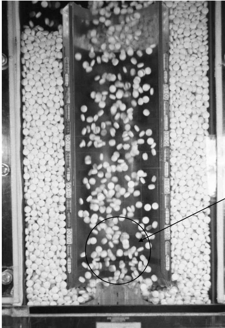
Figure A-17.2 Photograph of the fluidized bed at low gap height (2.7 cm) and modified deflector 1.
