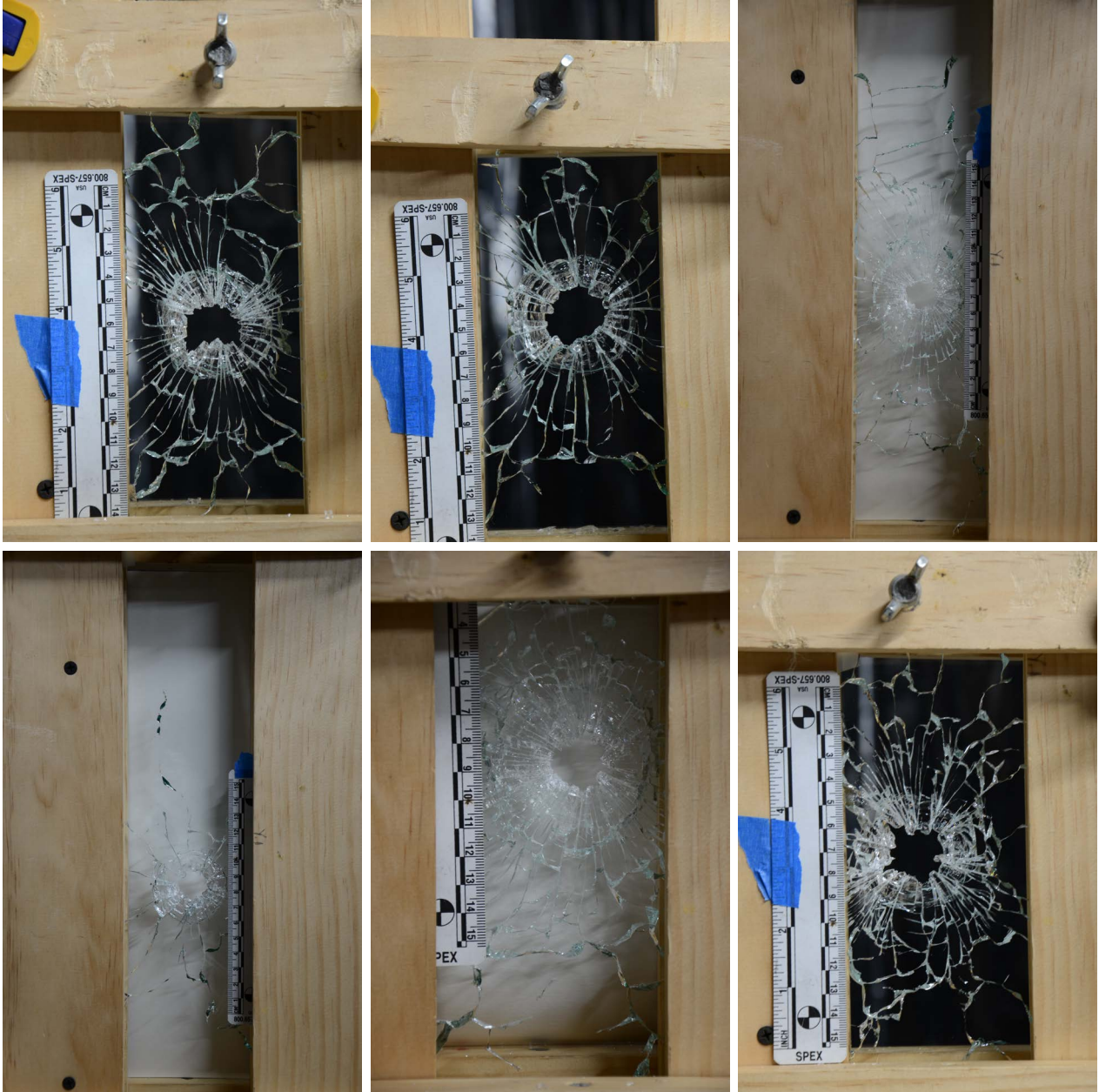
Figure 4.19: 60° full metal jacket bullet holes in glass. (Top row): 1A, 1B, 4I, (Bottom row): 4J, 5D, 8H
