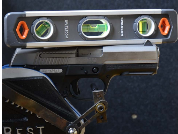
Figure 3.4: Process to ensure firearm is level in the vice
