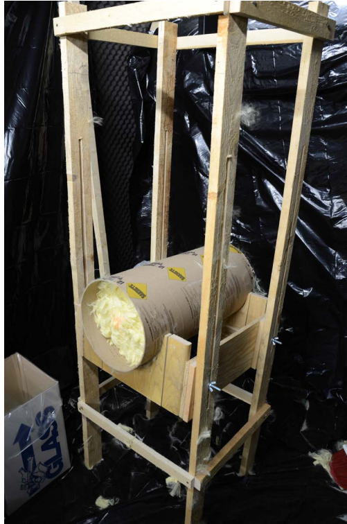
Figure 3.3: Kevlar ® bullet trap holder device
