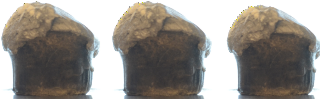
Figure 3.20: Measuring 5 (left), 10 (middle), and 15 (right) points on a 60° bullet using method HH.
