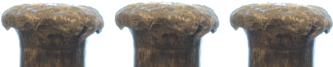
Figure 3.17: Measuring 5 (left), 10 (middle), and 15 (right) points on a 90° bullet using method HH.
