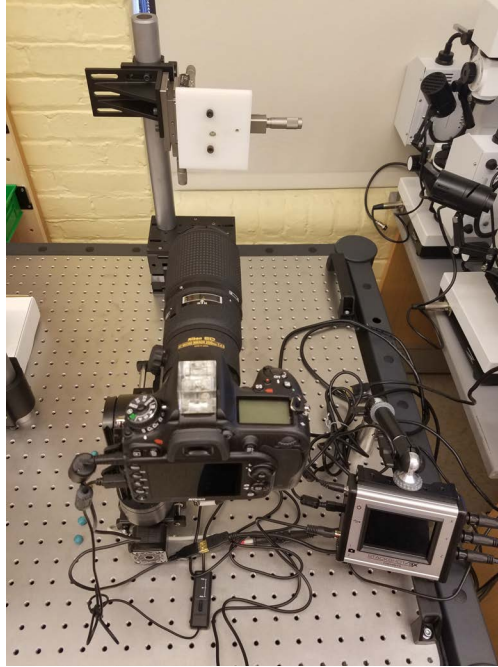
Figure 3.21: Focus stacking setup with Stackshot 3X TM
