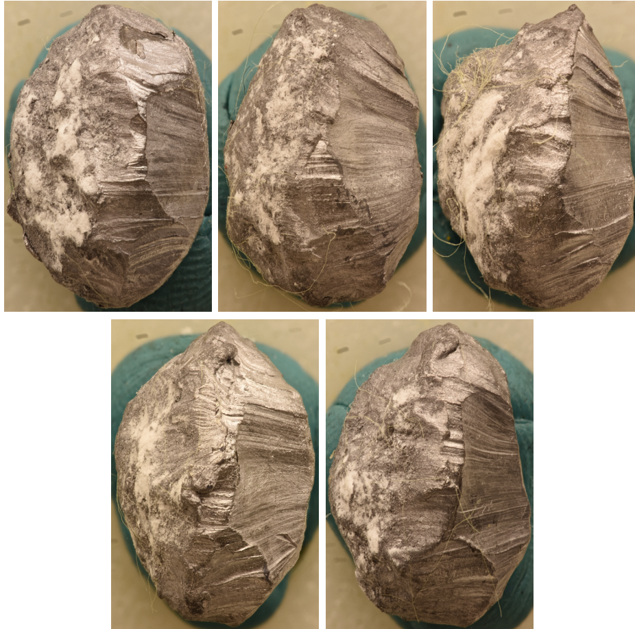
Figure 4.60: 45° problem bullets - samples 3B (top left) and 3K (top right); other 45° bullets - samples 1Q (bottom left) and 1W (bottom right)
