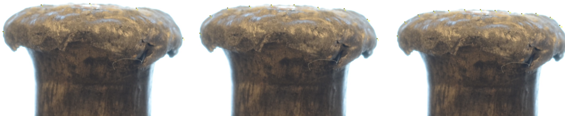
Figure 3.15: Measuring 5 (left), 10 (middle), and 15 (right) points on a 90° bullet using method AA.
