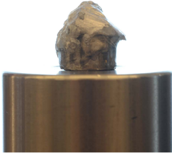
Figure 4.6: Bullet fired at 45° viewed from the side
