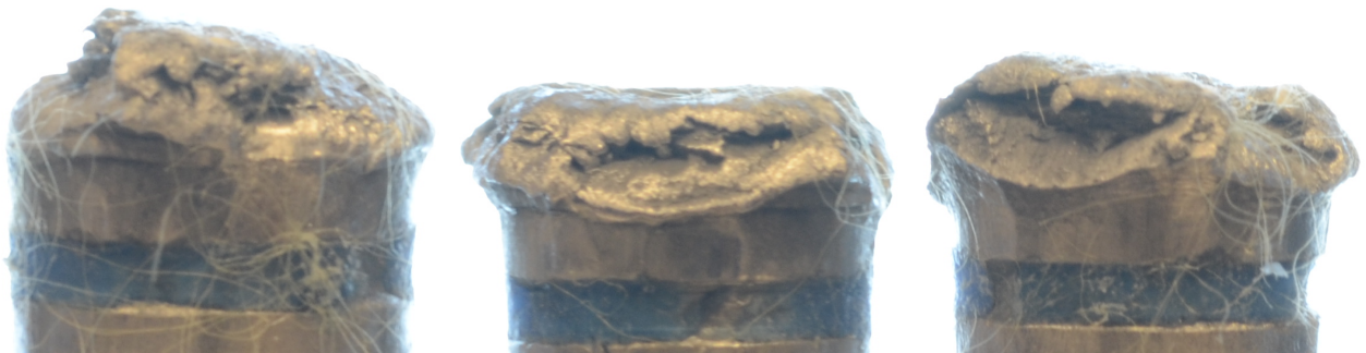
Figure 4.51: 90° problem bullet - Sample 5V (left); other 90° bullets - sample 5S (middle) and sample 5F (right)
