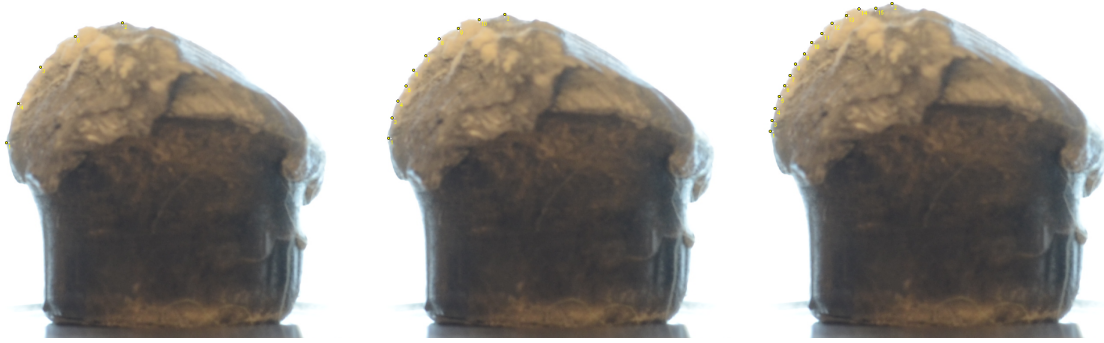
Figure 3.18: Measuring 5 (left), 10 (middle), and 15 (right) points on a 60° bullet using method AA.
