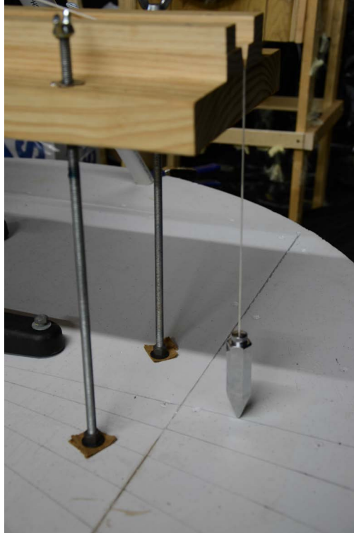
Figure 3.5: Plumb bob measuring the proper angle
