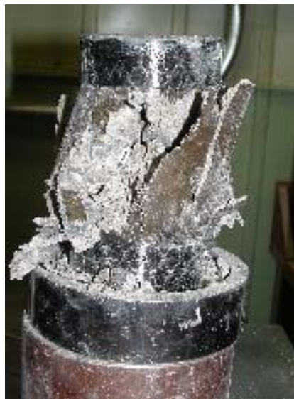
Figure 5-43 Failure in Specimen with 1” Height Wrap only at Top and Bottom
