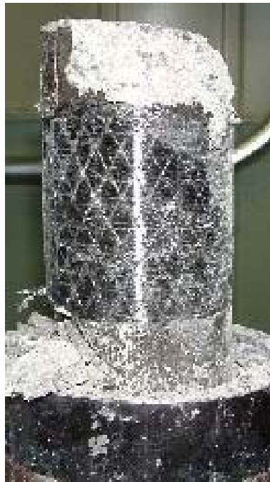
Figure 5-41 Failure in Specimen with 1½" Height Gap (Top and Bottom)
