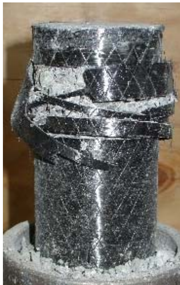
Figure 5-30 Failure in One layer FRP Wrapped 3"x 6" Specimen
