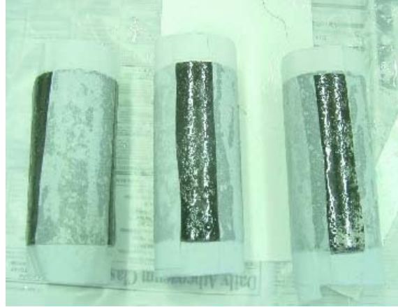
Figure 4-15 Wrapping of Parchment Paper on the Resin Coated Specimen
