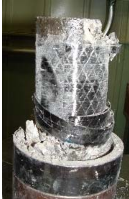
Figure 5-40 Failure in Specimen with 1" Height Gap (Top and Bottom)
