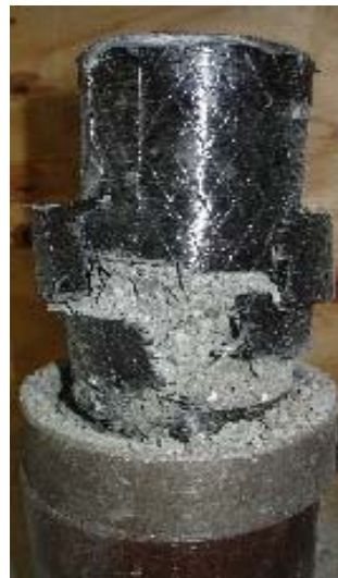
Figure 5-32 Failure in Six Layer FRP Wrapped 3"x 6" Specimen
