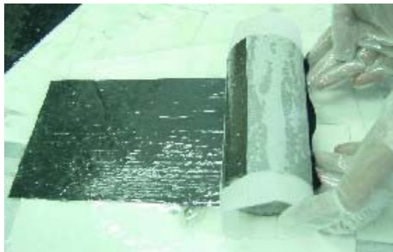
Figure 4-16 Wrapping the Resin Coated Fiber on the Parchment Paper Wrapped Specimen
