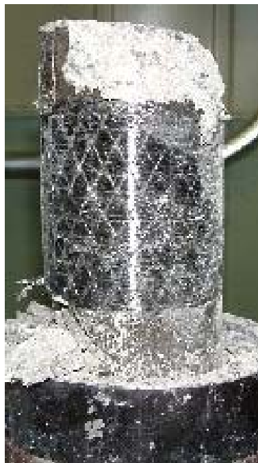
Figure D- 1 Partially Wrapped Specimen – Failure Pattern
