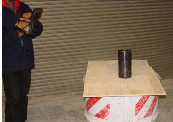
Figure 4-19 Infrared Thermography Tests: Along the Circumference of the Wrapped Cylinder
