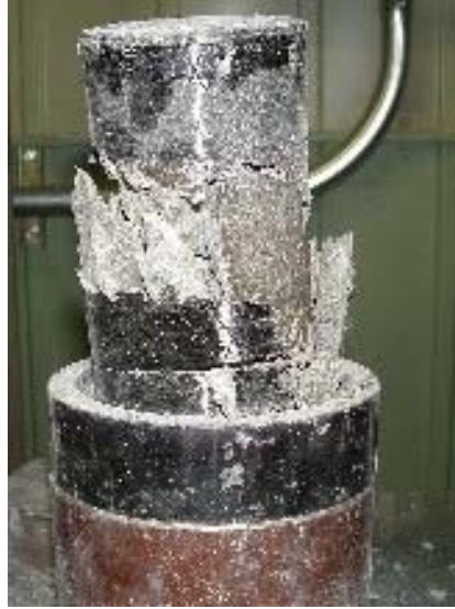
Figure 5-42 Failure in Specimen with 1½” Height Wrap only at Top and Bottom
