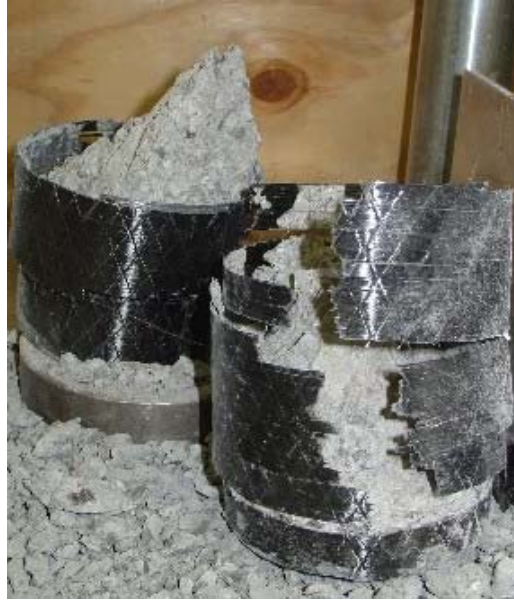
Figure 5-31 Failure in Three layer FRP Wrapped 3"x 6" Specimen
