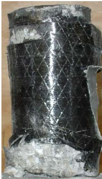
Figure 5-39 Failure in Specimen with ½" Height Gap (Top and Bottom)
