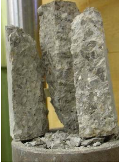
Figure 5-29 Failure in Non Wrapped 3"x 6" Specimen
