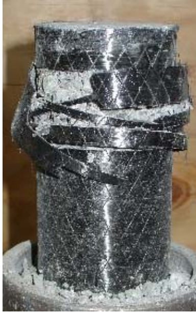
Figure 5-38 Failure in Completely Wrapped Specimen
