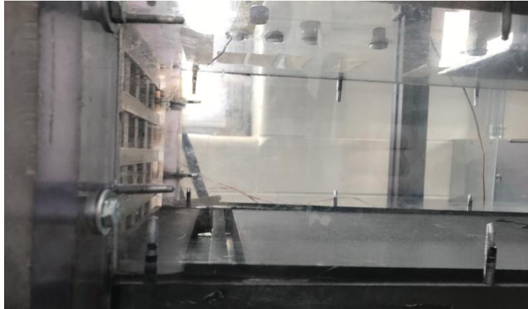
Figure 43 - Suction Slots and Test Region without Probes
