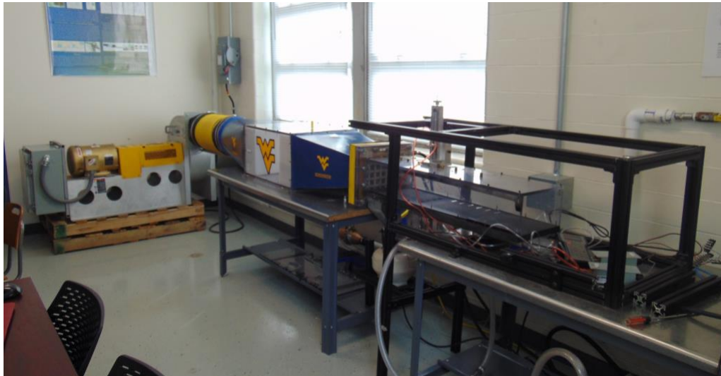
Figure 31 - WVU Subsonic Wind Tunnel at Test Section Exit
