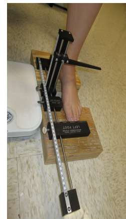
Figure 2: Arch Height Index Measurement System
