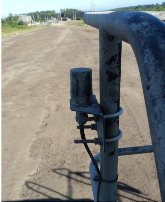
Figure 2.26 Radio antenna mounted on hand rail of dump truck
