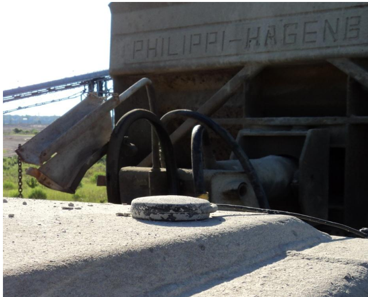
Figure 2.27 GPS receiver mounted over operator's cabin
