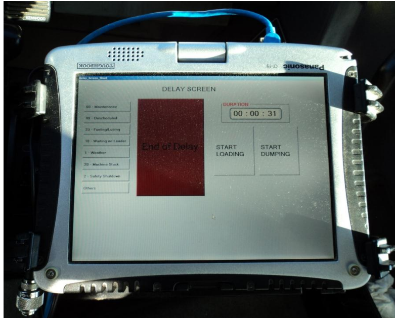
Figure 2.24 On-board touch-screen personal computer
