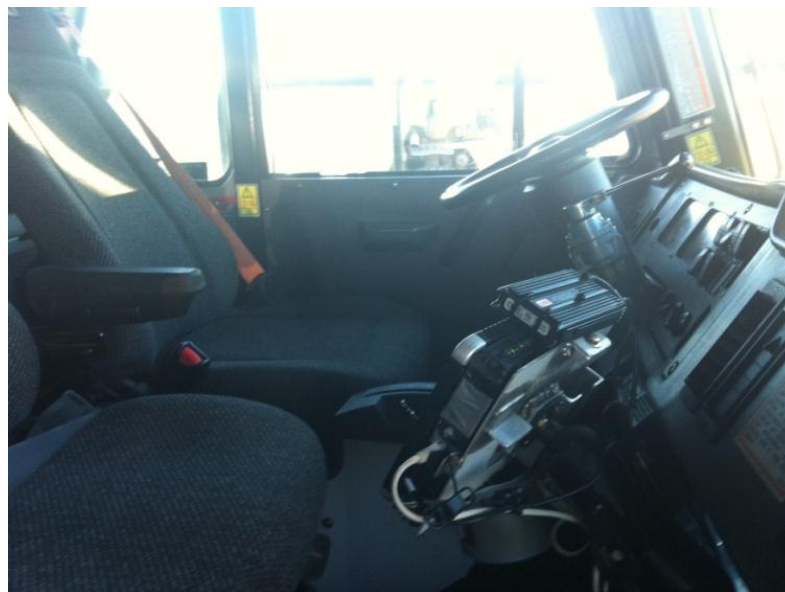
Figure 2.25 On-board computer mounted in dump truck cabin
