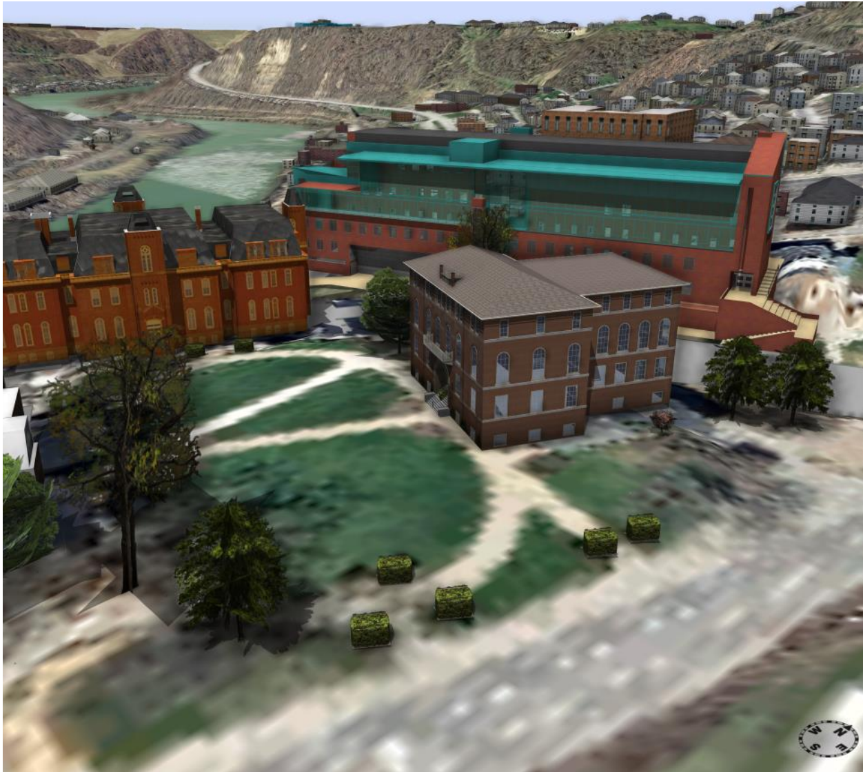
Figure 4-2: SketchUp models used within CityEngine to create WVU's historic Woodburn Circle, with Sunnyside, the Monongahela River, and Evansdale in the background. The building models were placed manually on the terrain due to their individual orientations and small number. Street furniture and vegetation were located through procedural rules due to their larger quantity and lesser need for high detail. The buildings in Sunnyside are mostly procedurally generated as houses or apartment buildings.
