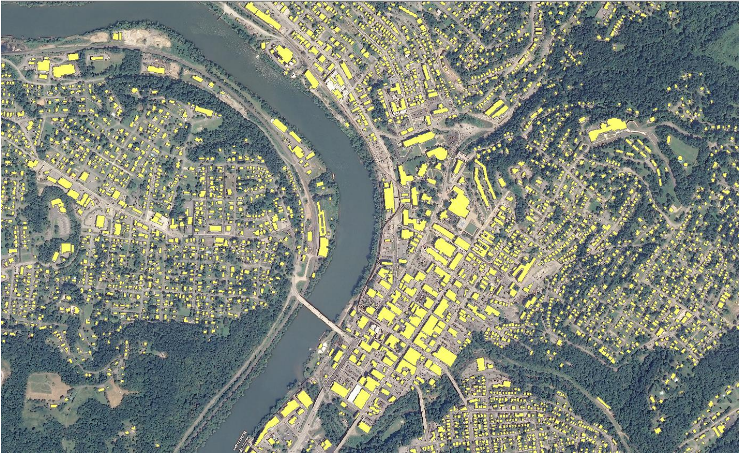
Figure 4-1: City of Morgantown 2D building footprint shapefile draped over three-foot NAIP imagery within ArcGIS. The shapefile attributes included land use and maximum building height, both of which were identified and used within the procedural rules of CityEngine for extruding and rendering the built environment.
