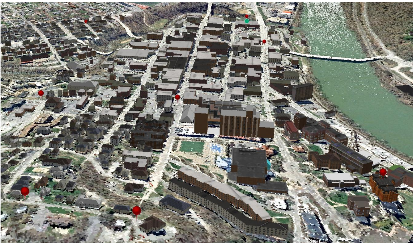
Figure 4-10: Observer points (red pins) placed for the sight line creation phase of intervisibility analysis.
