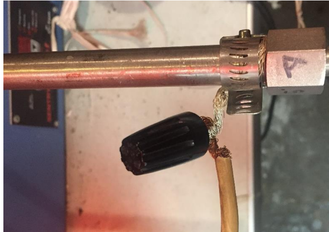
Figure 3.7 Load cell securely connected to end of manifold using wire nuts and clamps.
