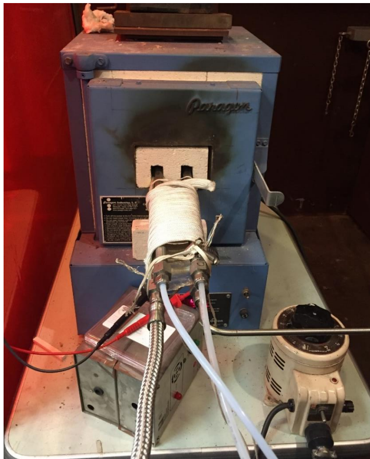
Figure 3.8 Manifold assembly loaded into the furnace with fuel lines connected. The weights used to apply pressure onto the stack, heating tape, and voltage measuring leads are also visible.
