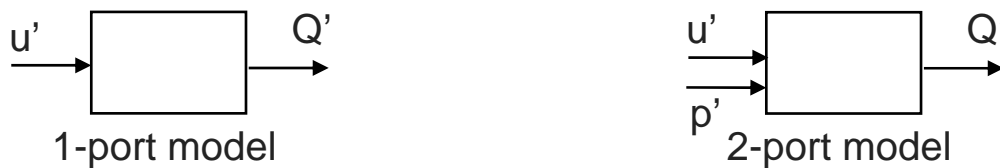
Figure 4.3: Burner / flame characterization as an (a) active acoustic one-port or (b) active acoustic two-port.
