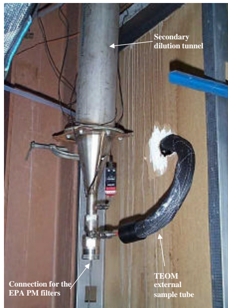
Figure 11: The TEOM sampling location on the secondary dilution tunnel
