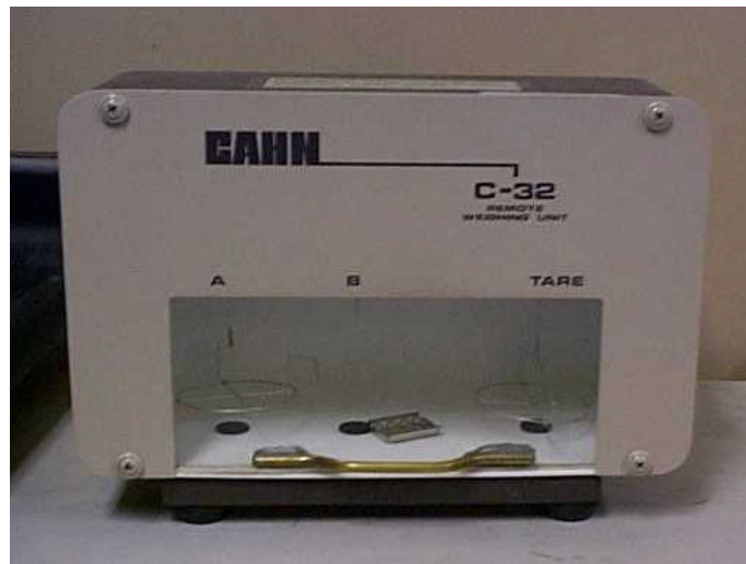
Figure 7: The microbalance used weigh conventional PM filters before and after each test.
