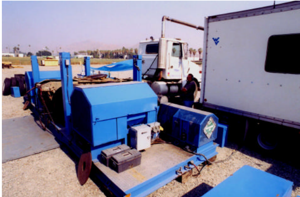
Figure 13: Although this illustration does not show the transit busses used, illustrated here is a typical vehicle operation on the portable heavy-duty chassis dynamometer.
