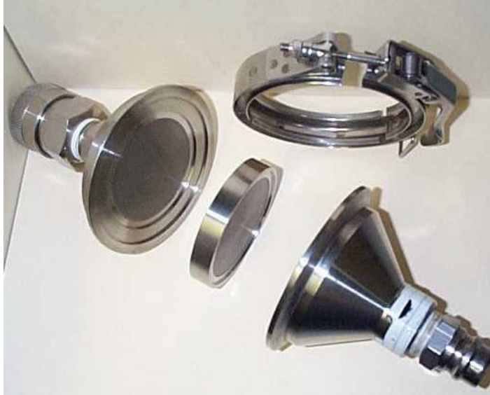
Figure 4: The 70 mm diameter PM filter cartridge disassembled. This filter module was used for the conventional, EPA-style, PM collection.
