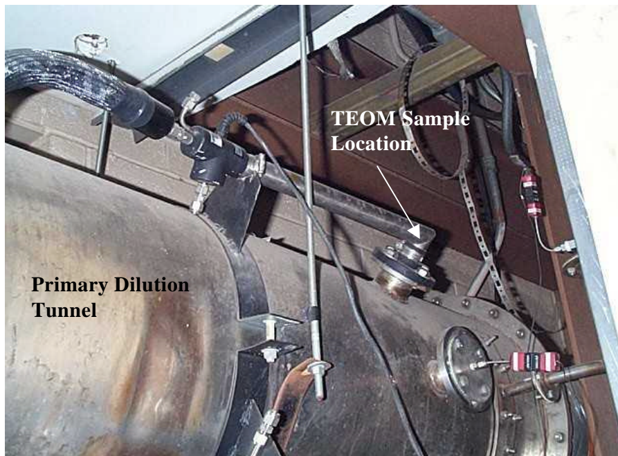
Figure 9: The TEOM sampling location on the primary dilution tunnel.
