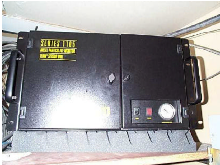
Figure 16: The front panel of the TEOM. Although the results were not verified, the foam that the TEOM was resting upon was to help eliminate external vibration.
