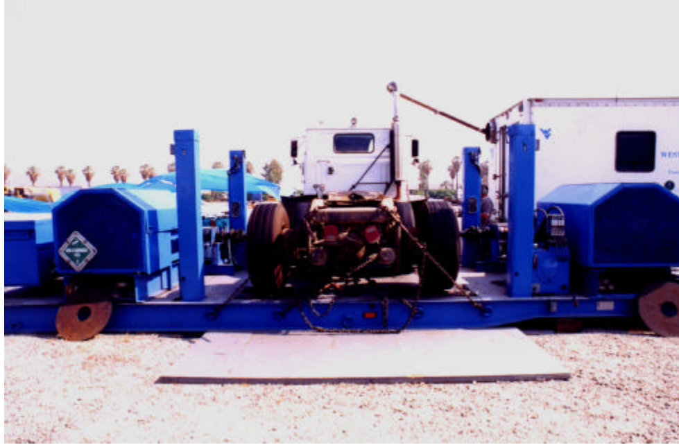
Figure 14: Typical routing of vehicle exhaust into the emissions trailer of the mobile laboratory.
