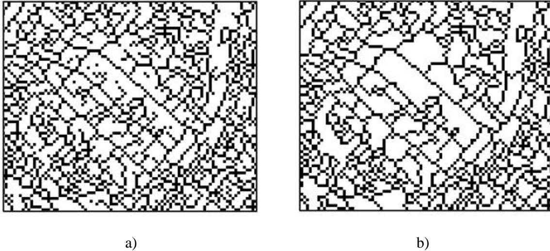
Figure 3-8. The results of the thinning and pruning process. a) Skeletonized image after thinning process, and b) Image after pruning process for a part of the study area. (Compare with Figure 3-7.)
