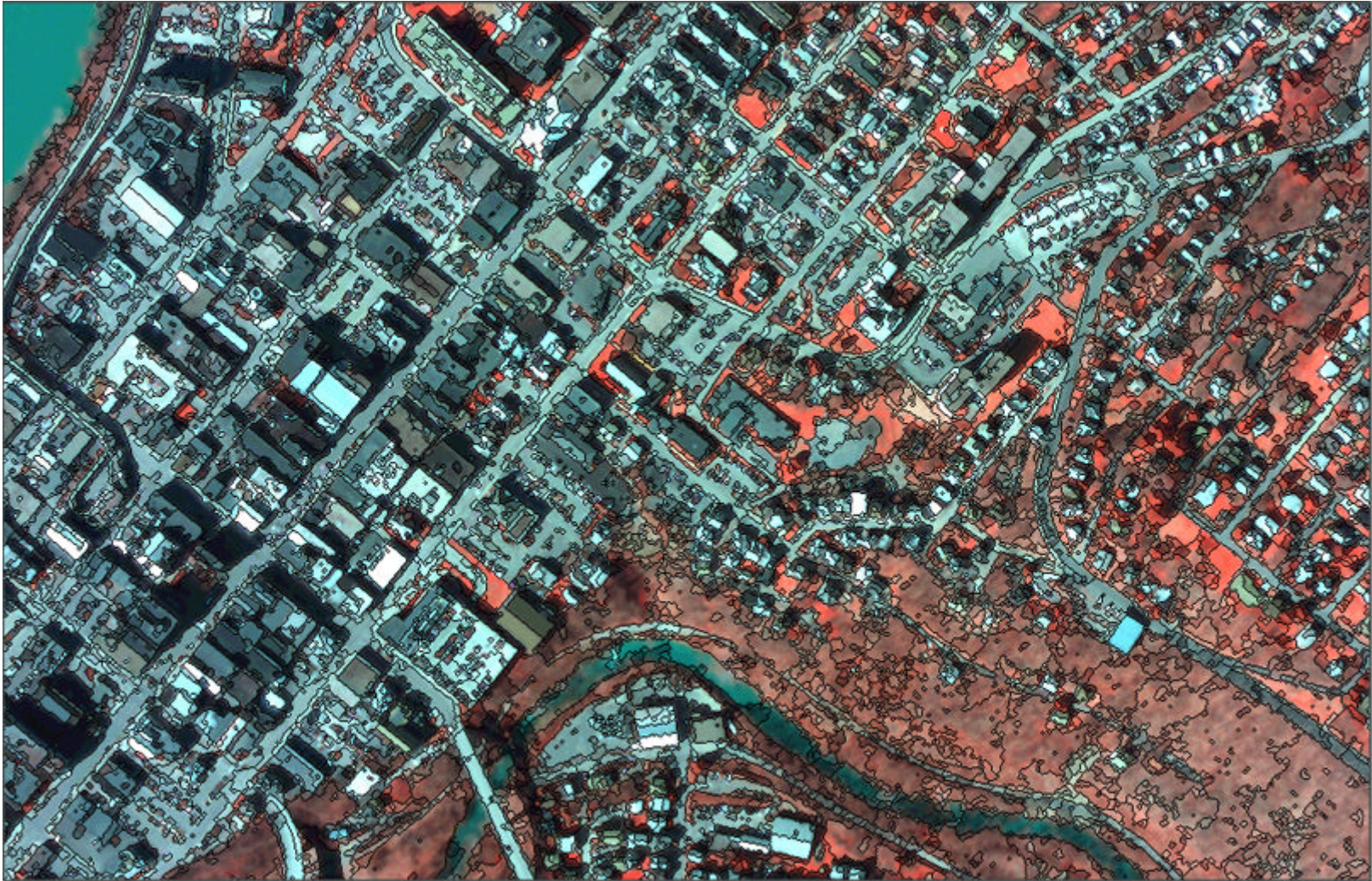
Figure 4-8. Patches produced by region growing with a significance level of 0.0005.
