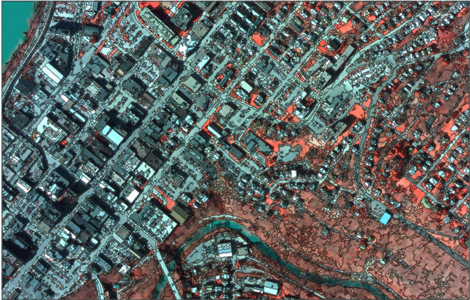
Figure 4-5. Image segments of sub-patches modified by vegetation edges.
