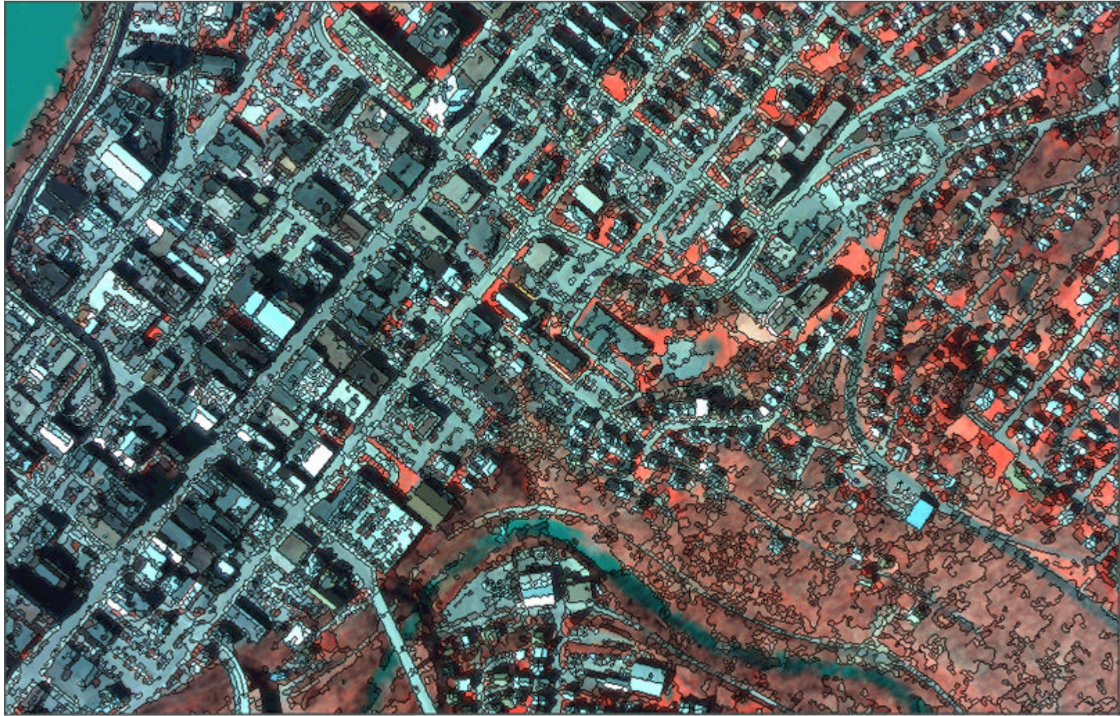
Figure 4-3. Image sub-patches delineated by an edge enhancement threshold level of 70.
