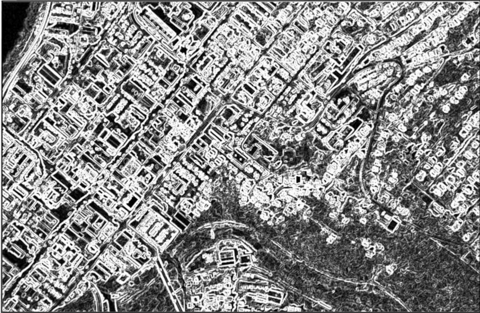
Figure 3-6. Edge enhancement of Morgantown ADAR data for a subset of the study area, including downtown and parts of the neighboring suburbs.
