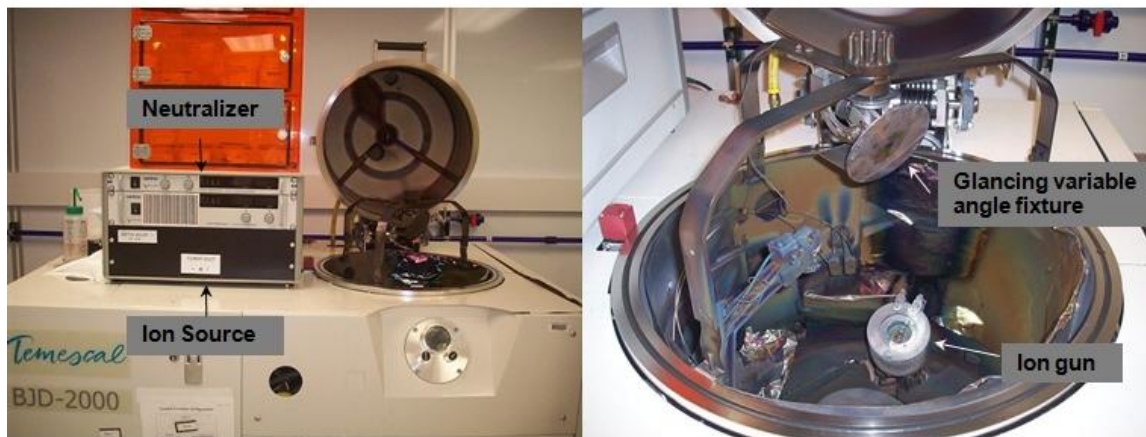
Figure 4-6 : (left) Electron beam evaporator, Ion beam assisted deposition equipment, and Glad fixture, (right) planetary was completely removed and replaced it with GLAD apparatus.
