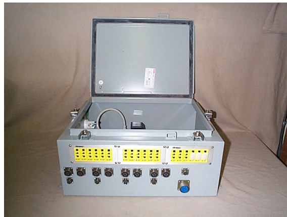
Figure 3-3 Datalogger with Top Open
